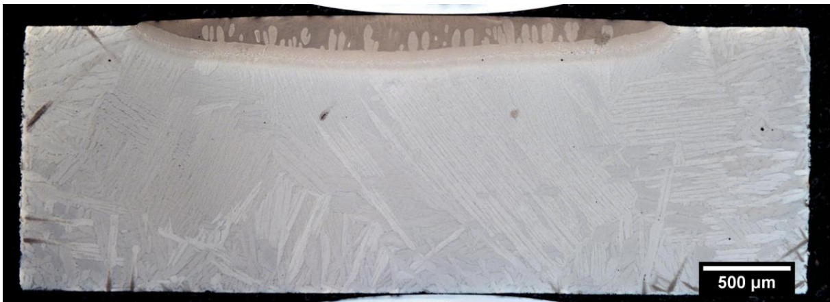
Figure 4.13 – Optical Imaging of Microstructural Cross Section of Ti-Cu Sample Heated to 1050°C and Cooled at 20 Kpm Showing Entire Width
