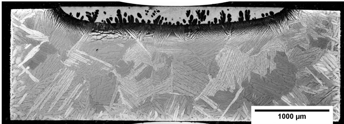
Figure 5.13 - Optical Imaging of Microstructural Cross Section of Ti-Ni Sample Heated to 1050°C and Cooled at 20 Kpm Showing Entire Width
