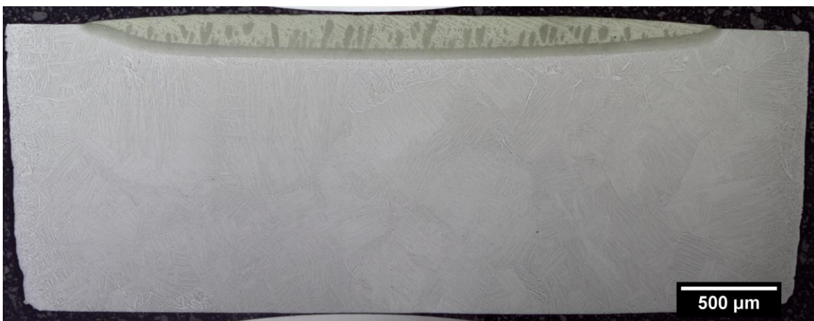
Figure 6.18 - Optical Imaging of Microstructural Cross Section of Ti64/Cu Sample Heated to 1050°C and Cooled at 20 Kpm Showing Entire Width
