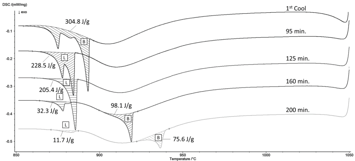
Figure 6.13 - Measurements of Cyclically Tested Sample Denoting Appropriate Use of Bezier (B) and Linear (L) Baseline Corrections
