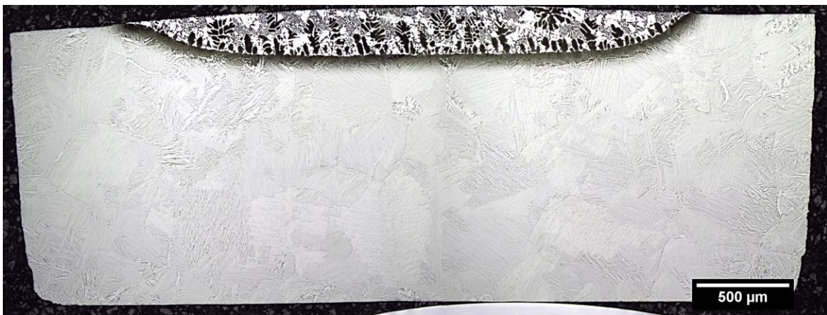
Figure 7.11 - Optical Imaging of Microstructural Cross Section of Ti64/Ni Sample Heated to 1050°C and Cooled at 20 Kpm Showing Entire Width
