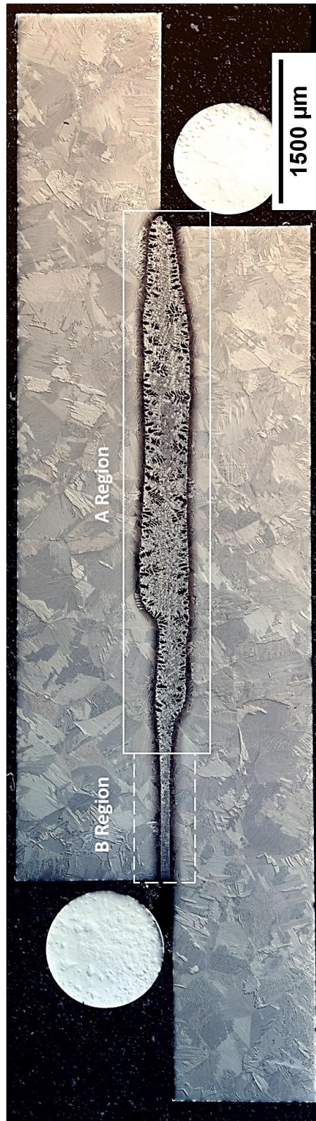
Figure 7.16 – Optical Imaging of Ti64/Ni/Ti64 DIL Sandwich Full Joint Heated to 1050°C and Cooled at 40 Kpm with Two Ni Foils
