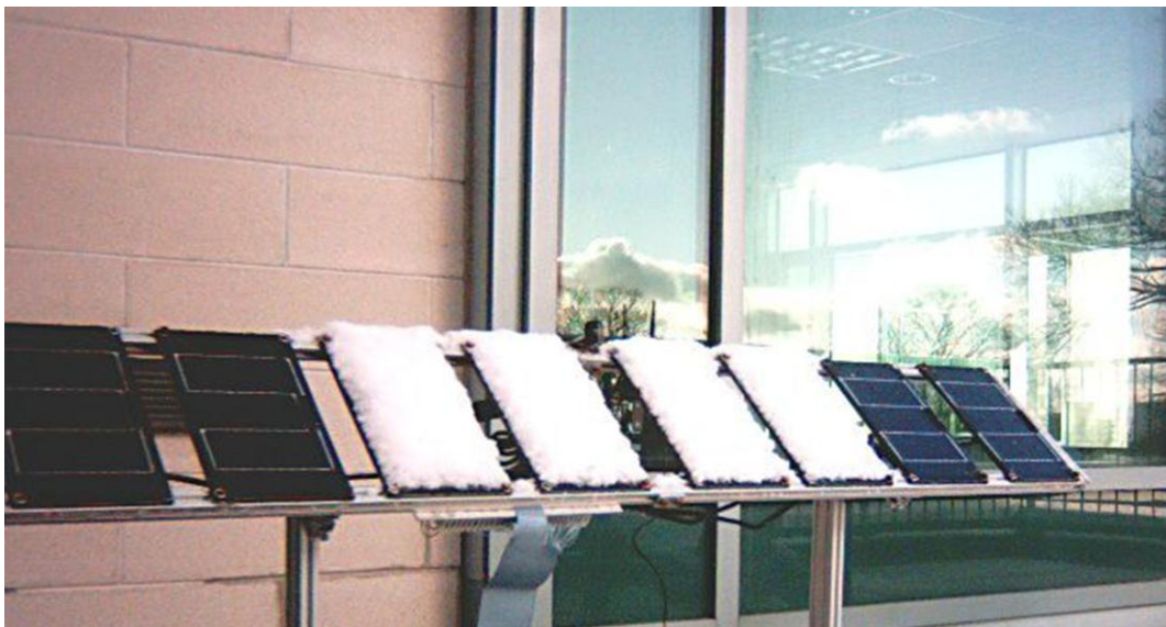
Control panels covered with snow; the snow on the treatment panels has been removed
