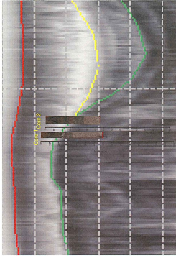
Figure 3.4 – Longitudinal seismic line showing general setting with an enlargement of seismic section surrounding cores 1 and 2. For this and following figures, the vertical scale is 10 ms = 7.5 m.
