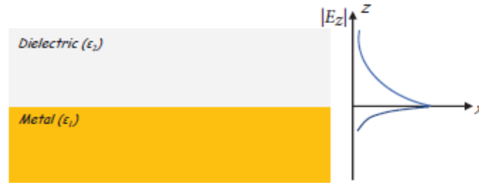
Figure 2.1 Schematic view of SPPs propagating along a single metal-dielectric interface
