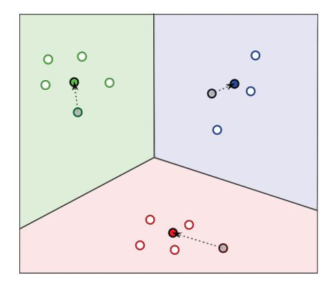
Figure 2.1: A potential k-means clustering, where the gray filled points are the initial centroids. The black outlined points are the final converged centroids, with their Vornoi partition shown and each point assigned to that centroid outlined in the same color.
