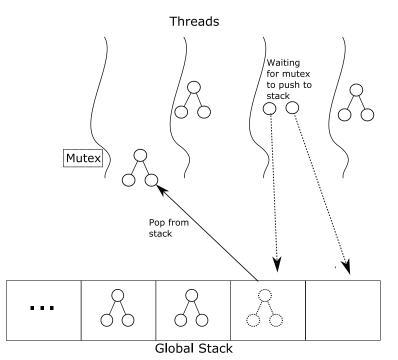
Figure 5.2: The global stack parallel filtering algorithm keeps a global stack for traversal order shared by all threads. Threads pop from the stack when they require more work, and push new work to the stack after they have processed a node. These operations are mutex protected to ensure the integrity of the stack and avoid work duplication leading to incorrect results.
