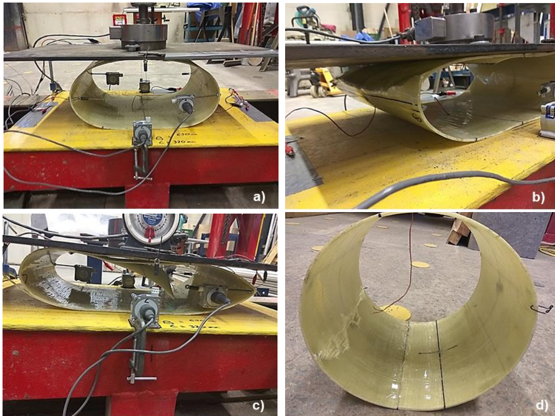
Figure 3: Modes of failure for GFRP liner (a) ring deflection; (b) cracking at springline; and (c) delamination at crown and wall buckling; and (d) regained shape after unloading
