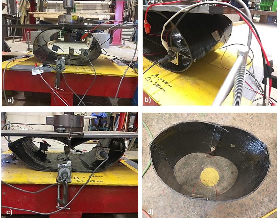
Figure 4: Modes of failure for CFRP liner (a) ring deflection; (b) cracking at springline; and (c) reversal of curvature at the crown and lift at invert; and (d) deformed shape after unloading
