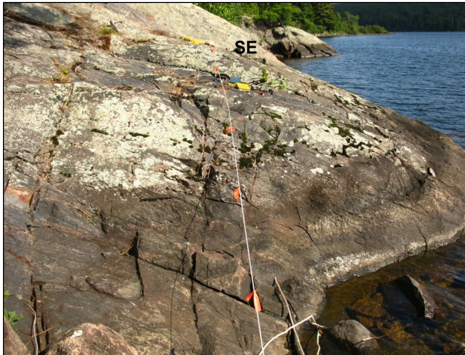
Figure 2.1: Baseline on a mylonitized migmatite. Flagging tape marks metre increments. Samples locations were then measured by the distance perpendicular to the baseline.
