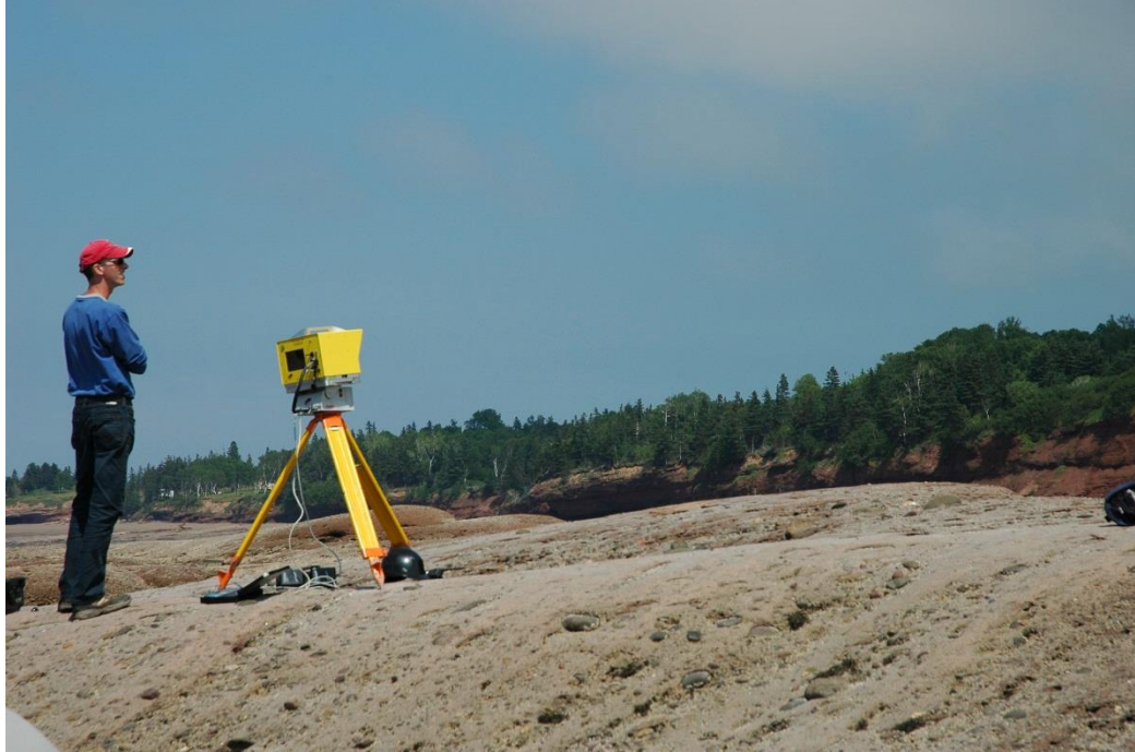
Figure 2.5 - Optech in. ILRIS HD lidar on a tripod, performing a scan (photo by Darragh O'Connor).
