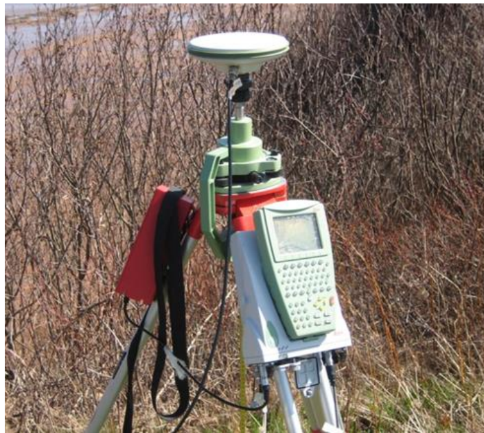
Figure 2.1 – DGPS base station (photo by Trevor Kelly).
