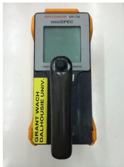
Figure 2.10 - Handheld Scintillometer, it measures the spectral gamma emission of the formation (K, U, Th)
