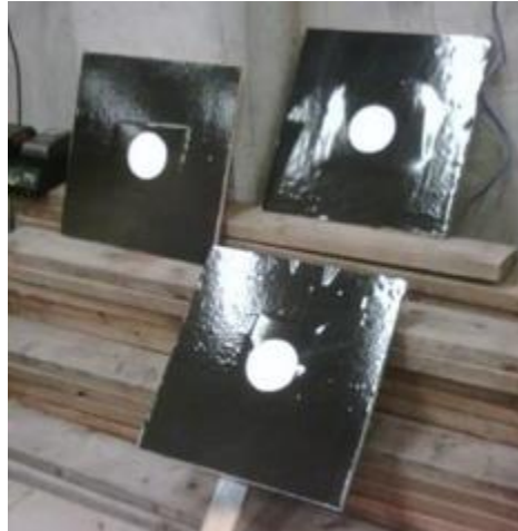
Figure 2.4 – Targets used for georeferencing. The targets have high reflective background (reflective black) contrasted with a less reflective centre circle, design by Johnathan Thibodeau.
