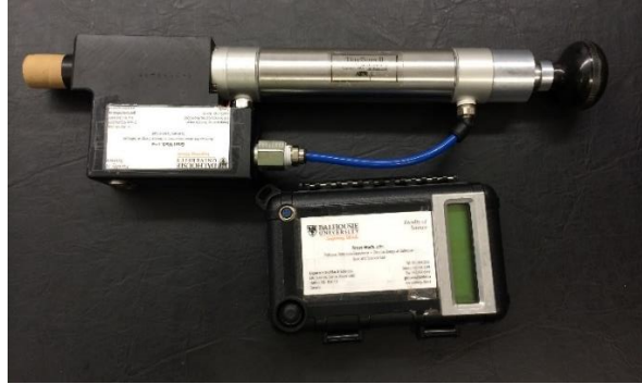
Figure 2.12 – Pneumatic device to measure permeability of the rock, in mD this is a TinyPerm II by New England Research Inc.
