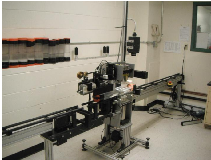
Figure 3.4. The Geotek Multi-Sensor Track (MST) Core Logger. This machine was used for spectrophotometer measurements, bulk density, p-wave velocity, magnetic susceptibility, high resolution photography and XRF measurements.
