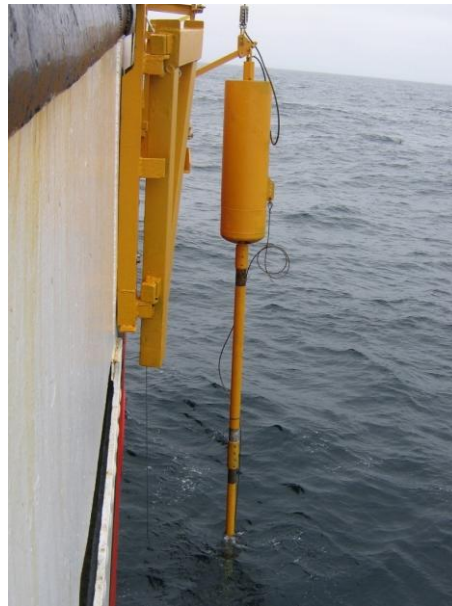
Figure 3.1. The piston corer on the CCGS Hudson. Photographed by Calvin Campbell, 2011.
