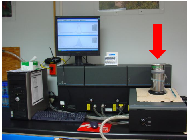
Figure 3.5. The Coulter laser in the GSC Sediment Laboratory. The sample, once mixed with water in a beaker, goes into the laser by pouring it into the column identified by the red arrow. Photographed by Owen Brown, 2012.
