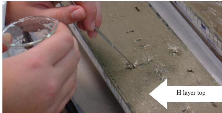
Figure 3.7. Close-up of the subsample being taken above a Heinrich layer shown in Figure 3.5. Photographed by Owen Brown, 2012.
