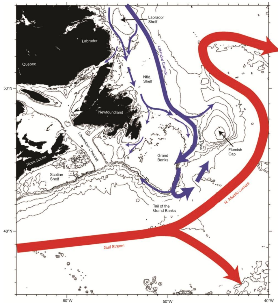
Figure 2.4. The Labrador Current is shown in blue, flowing southeastwards along the continental shelves and slopes of Labrador and Newfoundland. The Gulf Stream, transitioning to the North Atlantic Current as it splits, is shown in red. (Modified from Fratantoni & McCartney, 2010).
