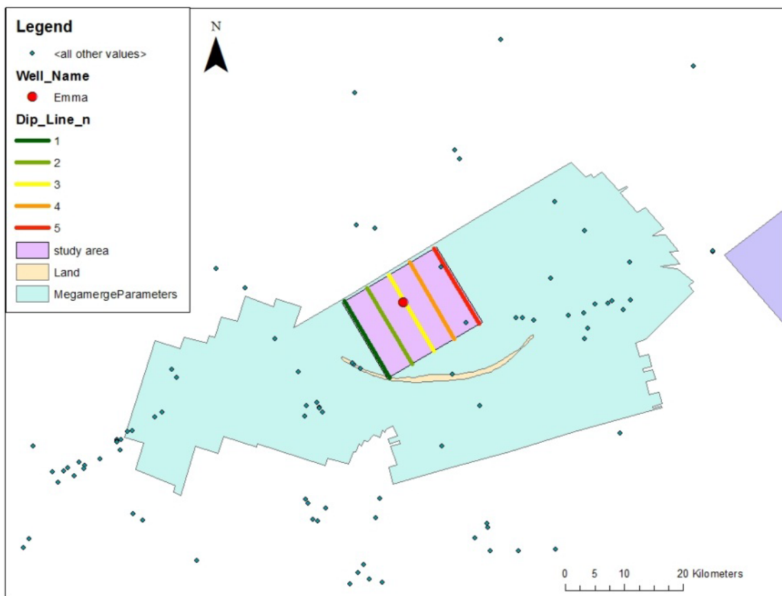
Fig. 2.1 Location of the five interpreted seismic lines and the one well with digital files available within the study area.
