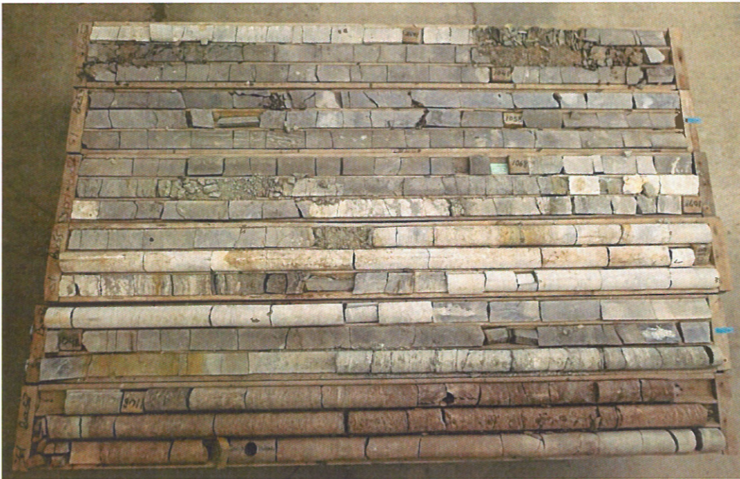
Figure 3-1 Photo of core from 1035-1120 ft depth. This photo shows the grey dolostone, the white (with minor blue) sulfate, and the red siltstone.
