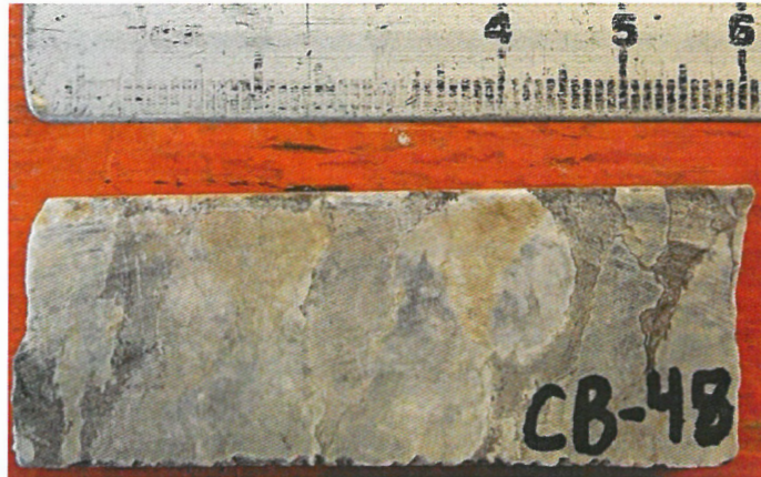
Figure 3-2 Photo of sample CB-48, a coarse nodular anhydrite with a silty dolostone matrix; ruler for scale with centimeters denoted.
