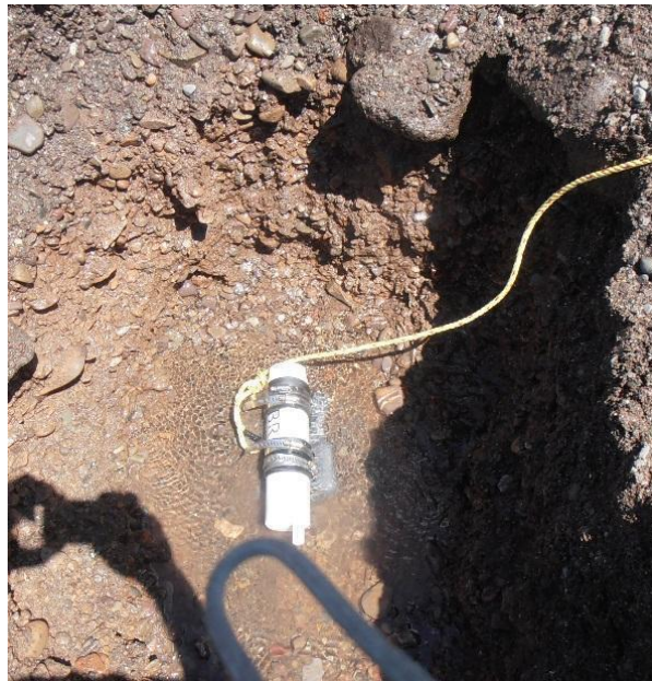
Figure 2.3 Installation of the Dalhousie pressure sensor near mid-beach at about 50 cm depth.
