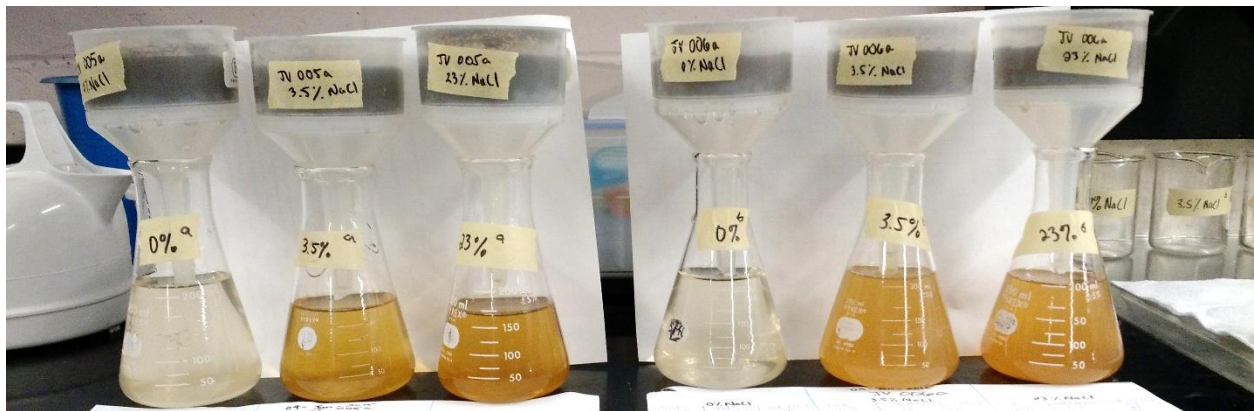
FIGURE 48 JV-005A AND JV-006A LEACHING EXPERIMENTS AFTER 600 ML OF SOLUTION
