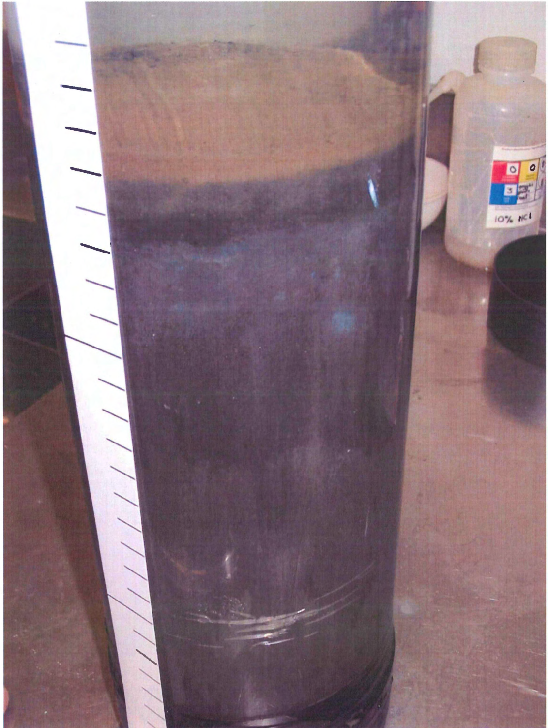
Figure 3.3 Photograph of a slow core collected from Halifax Harbour. Note the fine layer of reddish brown sediment at the top of the core, representative of the oxidized layer at the sediment-water interface which has been preserved through slow coring.
