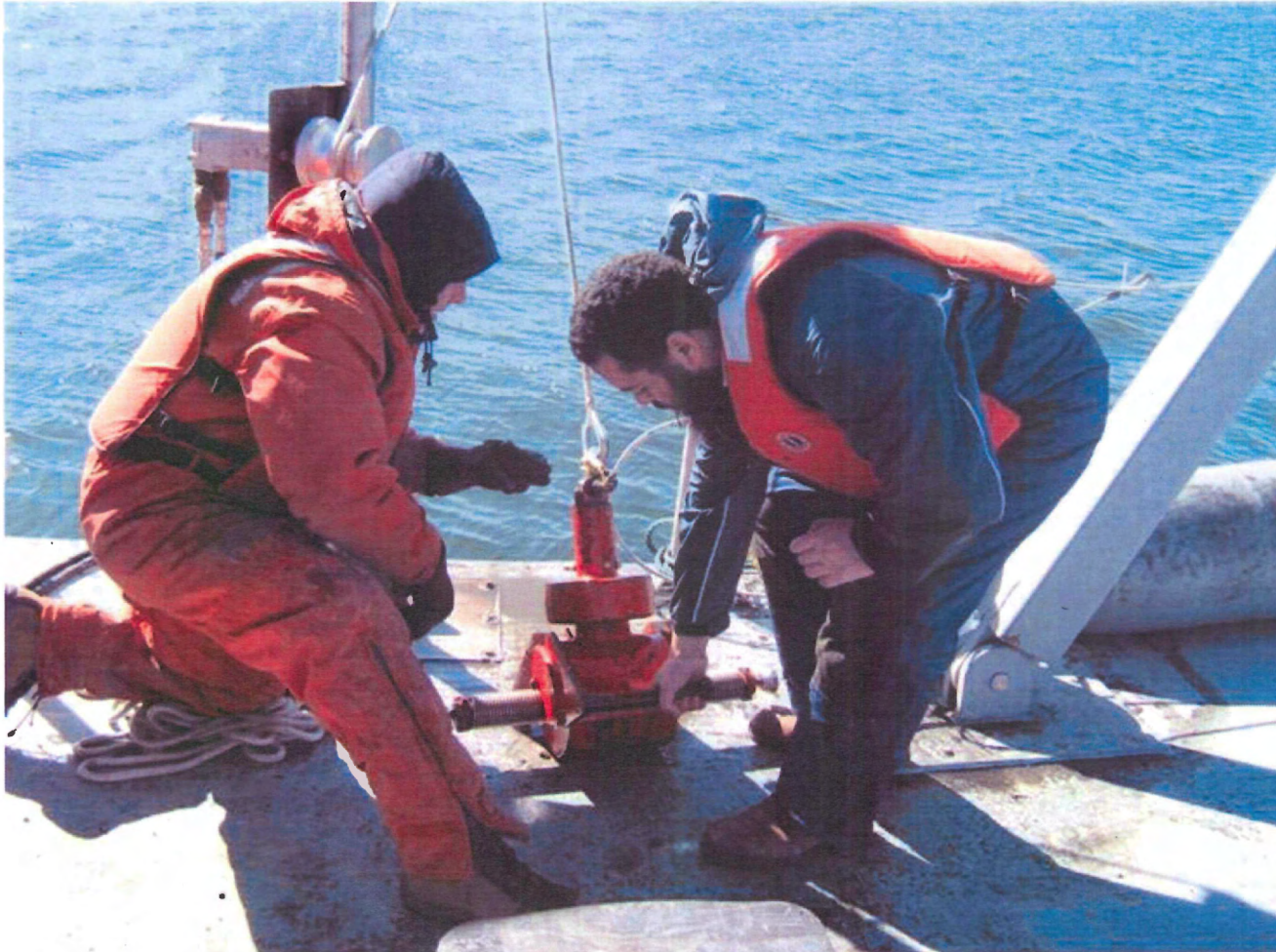
Figure 3.4 Photograph of a sediment grab sample being collected in Halifax Harbour using a Shipek grab sampler.
