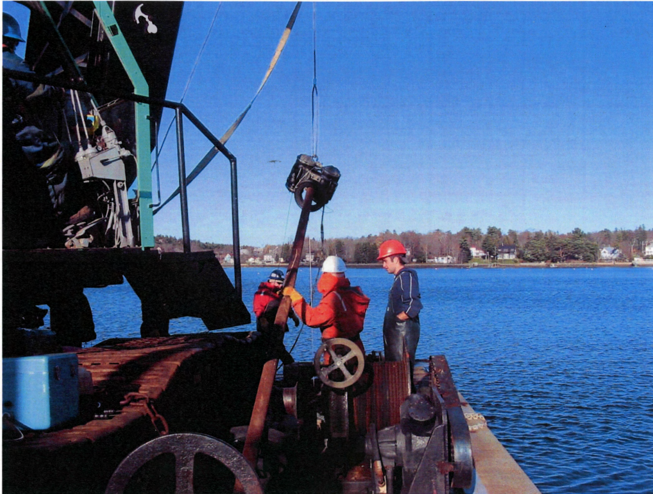
Figure 3.1 Photograph of a vibracore being collected in Halifax Harbour. Note the significant length of the core barrel, which allows cores as long as 6 m to be collected.
