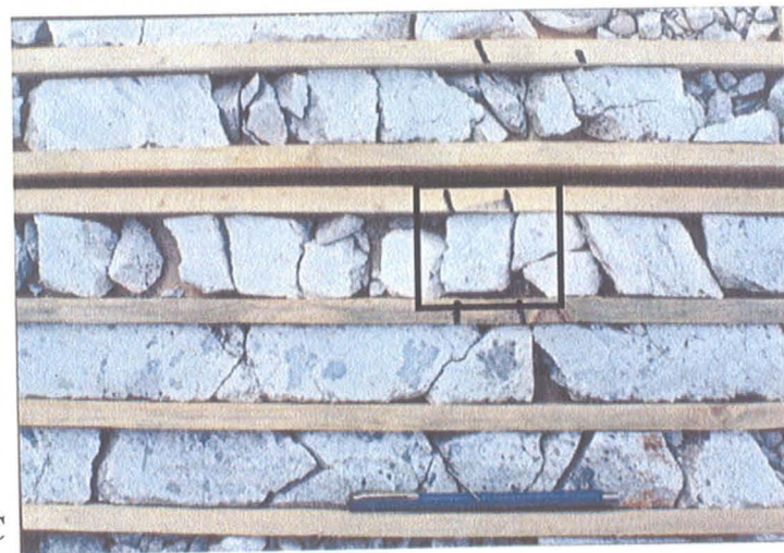
Figure 6.3. Photographs of DDH samples of background and albitised rhyodacites.
