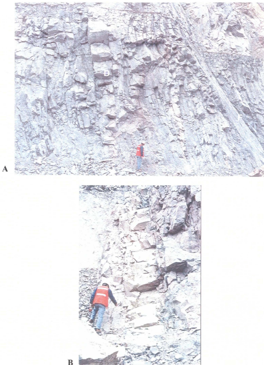
Figure 3.6. Photographs of rhyodacite flows and basaltic dykes at Morro open pit. A) Strongly developed columnar jointing in mineralised rhyodacite unit. Primary porosity and the competent nature of the rhyodacite make it the most favourable host rock. Note the different style of fracturing in basaltic dyke (D), and steep fault plane (F). Height of the bench is 12.5 m. B) Vertical basaltic dyke intruding rhyodacite. Most of these dykes are barren even though hydrothermal alteration and Cu mineralisation are usually strong within the volcanic country rocks adjacent to their contacts.
