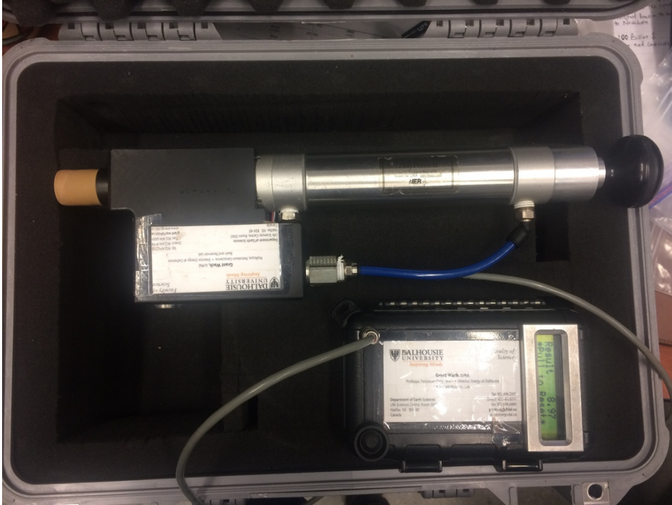
Figure 3.8. TinyPerm II handheld permeameter and data reporting screen from New England Research.
