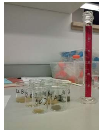
Figure C.2 Adding 4 mL deionized water into 200 mg samples for mounting two slides each sample
