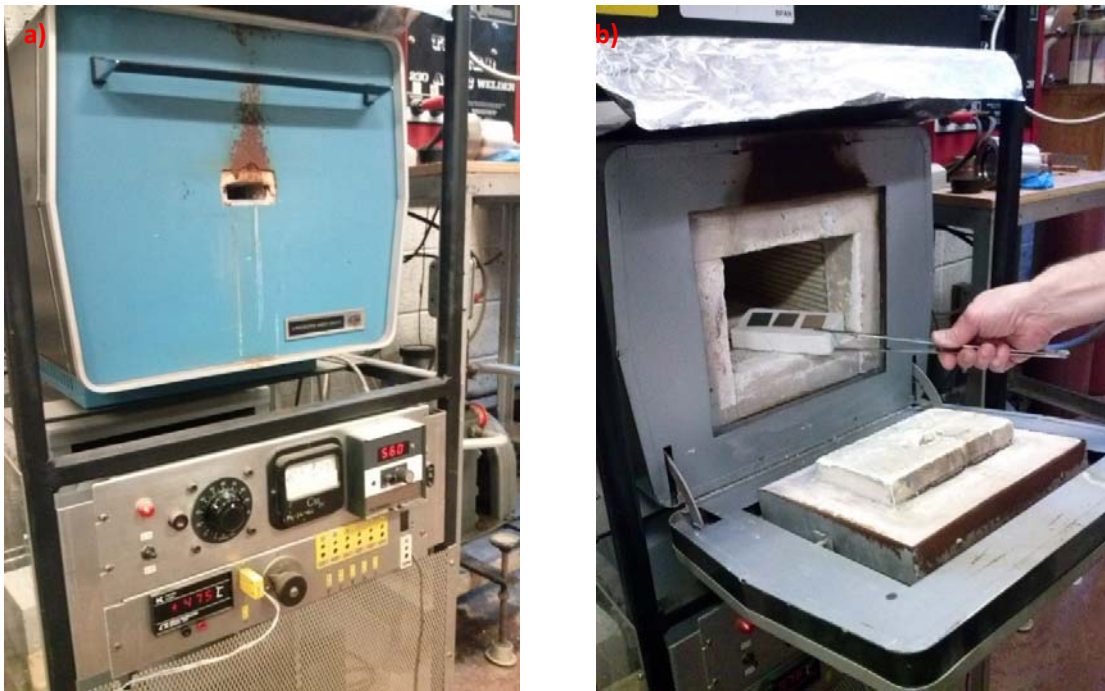
Figure C.8 a) Setting up the oven at ~550°C; b) Taking out slide samples after an hour.
