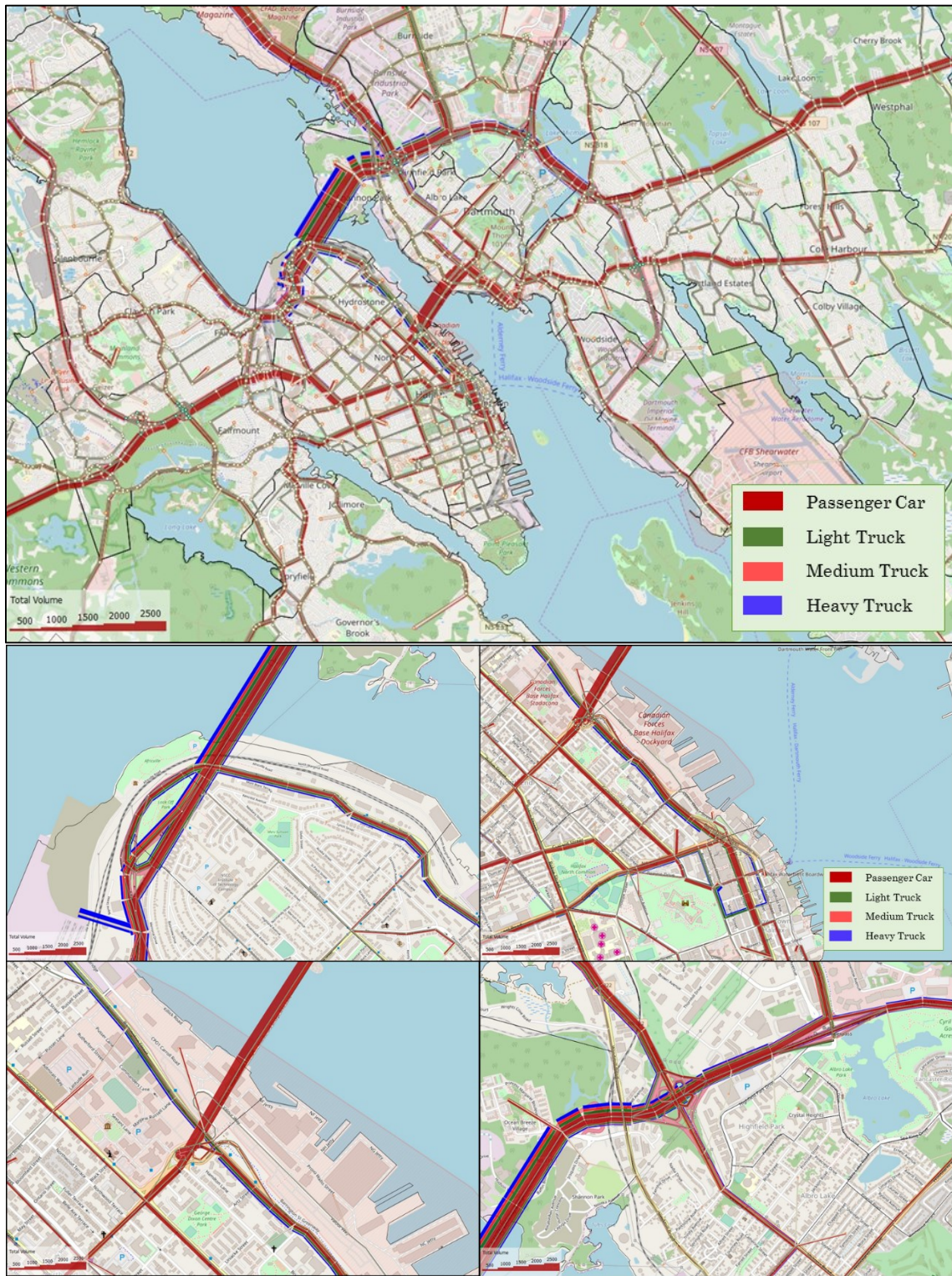
Figure F-1 Traffic Flow at Evening Peak Period in Transport Network Model
