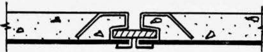
DETAIL OF BACK AND FRONT VERTICAL JOINT OF COPING, ALSO EXPANSION JOINT OF BUILDING UNIT
