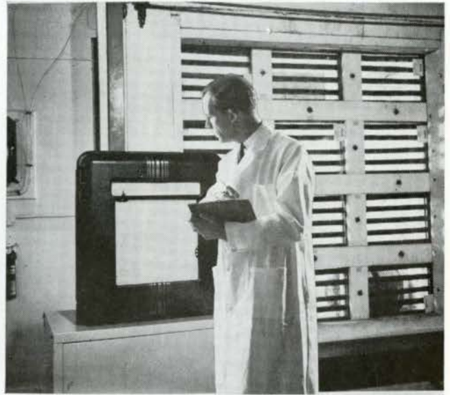
Technician checks temperature graph during accelerated weathering test.
