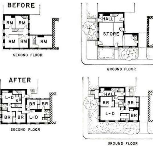
A successful conversion at Gore and Wellington streets. The original accommodation of eight rooms and a bathroom has been converted to one three bedroom and three two bedroom apartments. Architect, Selwyn Cooke.
