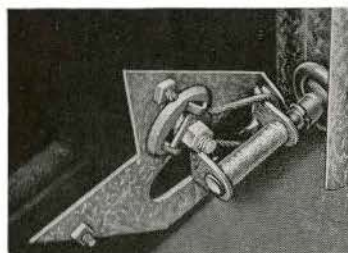
Bottom Roller Bracket with cable clamping device allows cable adjustment at floor level.
