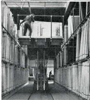
Over a quarter of a million square feet of Arborite (one of the many building materials) held in stock. Shown are full crates of Arborite, stored in new vertical racks for fast handling by a "guided" fork lift truck.
