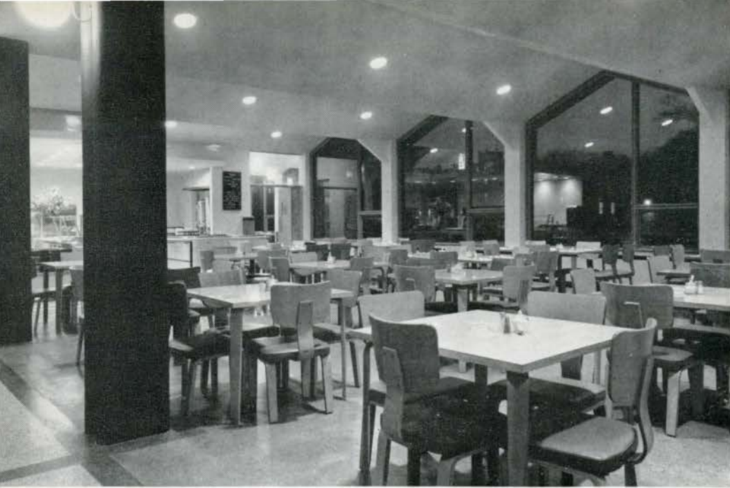
The cafeteria is used by the women undergraduates. Main illumination is provided by louvred fixtures recessed in acoustic plaster ceiling.
