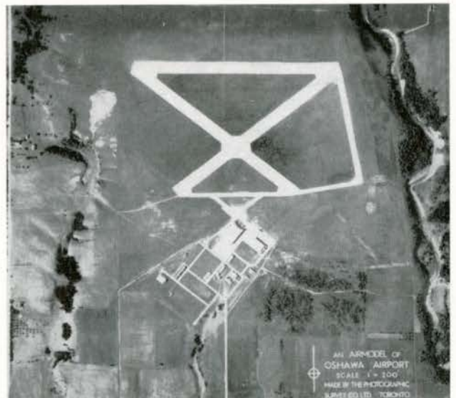
The accuracy now obtainable in topographical modelling is well illustrated by this illustration of the Airmodel of Oshawa Municipal Airport, made from air photographs.
