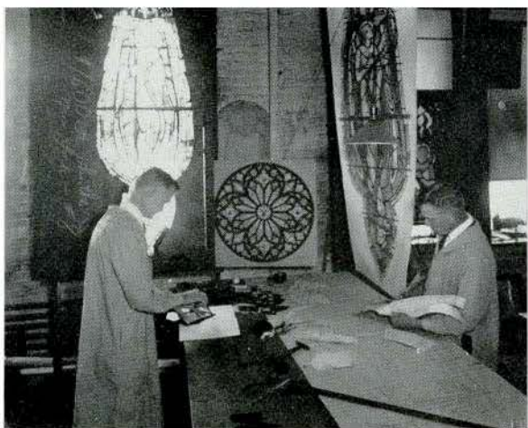
Glass being cut to patterns. In the background: a black-lined easel: the coloured design (in this case the Rose at the Cathedral of St. John the Divine, New York) and on the right, a cartoon of one section of the same window.
