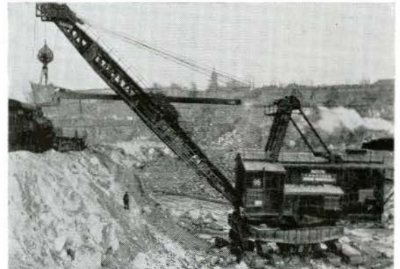
A GIANT POWER SHOVEL so big that it could hold a one-and-a-half storey house in its control cab, is shown loading ore cars with asbestos-bearing rock. The locomotive transports the ore to the J-M mill, which is located at the top of the pit.
