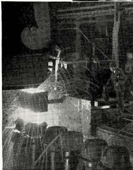
Jack McDonald watches "Basket Pouring," a delicate operation at the open hearth furnaces. In the production of certain special steels, the molten metal is poured through a steel box, into two ingot moulds simultaneously. This slows up the rush of steel into the mould, giving a better surface to the product. Gases escape and impurities rise to the surface, producing a cleaner steel.
