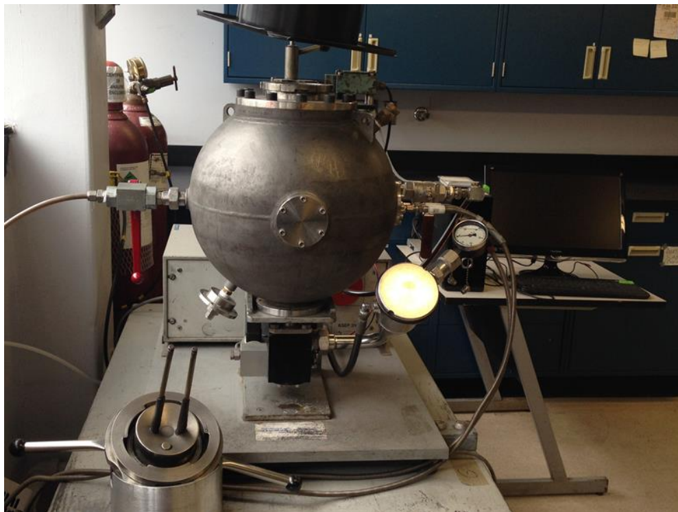
Figure 3.7: Photo of Siwek 20-L explosion chamber
