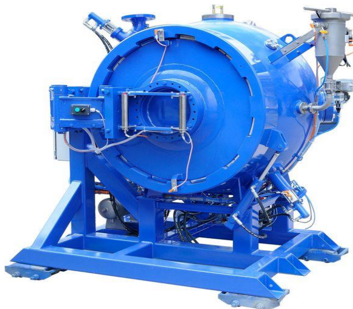
Figure 3.10: Photo of the Fauske and Associates Inc. 1-m 3 Explosion Chamber [50]
