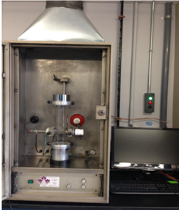
Figure 3.12: Photo of MIKE-3 apparatus
