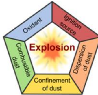
Figure 2.2: Dust explosion pentagon [5].
