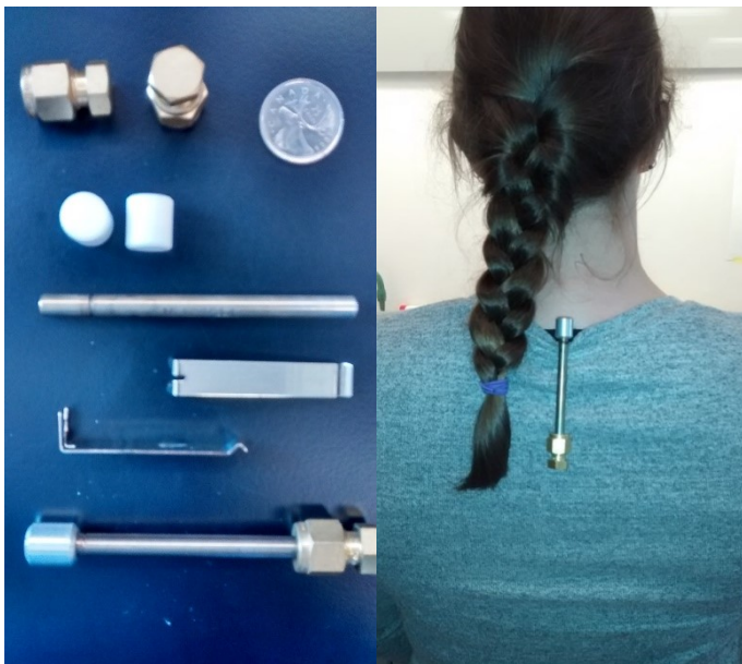
Figure 1. Thermal desorption sampling tools: A) Swagelok® caps to seal the tube airtight during transportation, 21g weight, B) white caps for use during short-term storage and chemical analysis, C) thermal desorption tube: metal cylinder 8.9cm by 0.5cm, 9g weight, D) metal clasp, E) sampling setup with filter on the left end, 32g total weight, F) wearing the tube at the back of the shirt.
