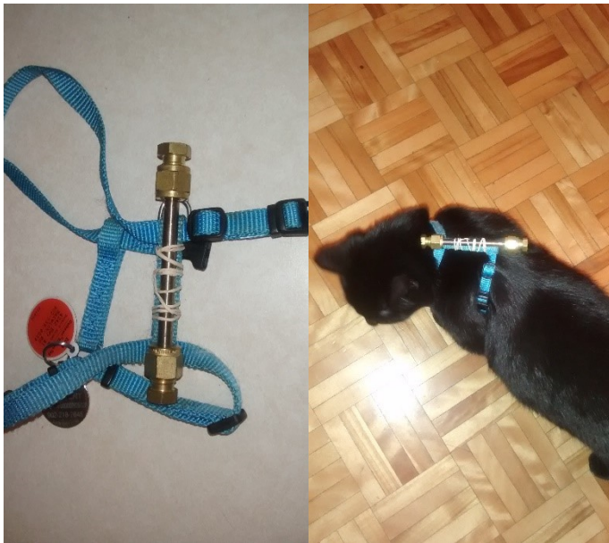
Figure 2. A) Thermal desorption tube attached to a feline halter, B) cat trained to wear a halter comfortably walking around the house.
