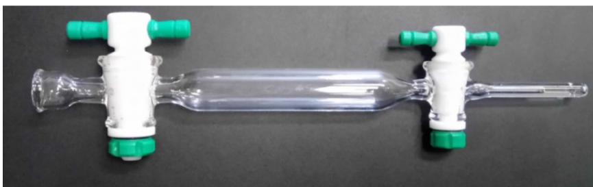
Figure 3.7: A device to deliver a constant volume of fluid to the viscometer. The volume between the two stopcocks is 11.00 \pm 0.03 mL.
