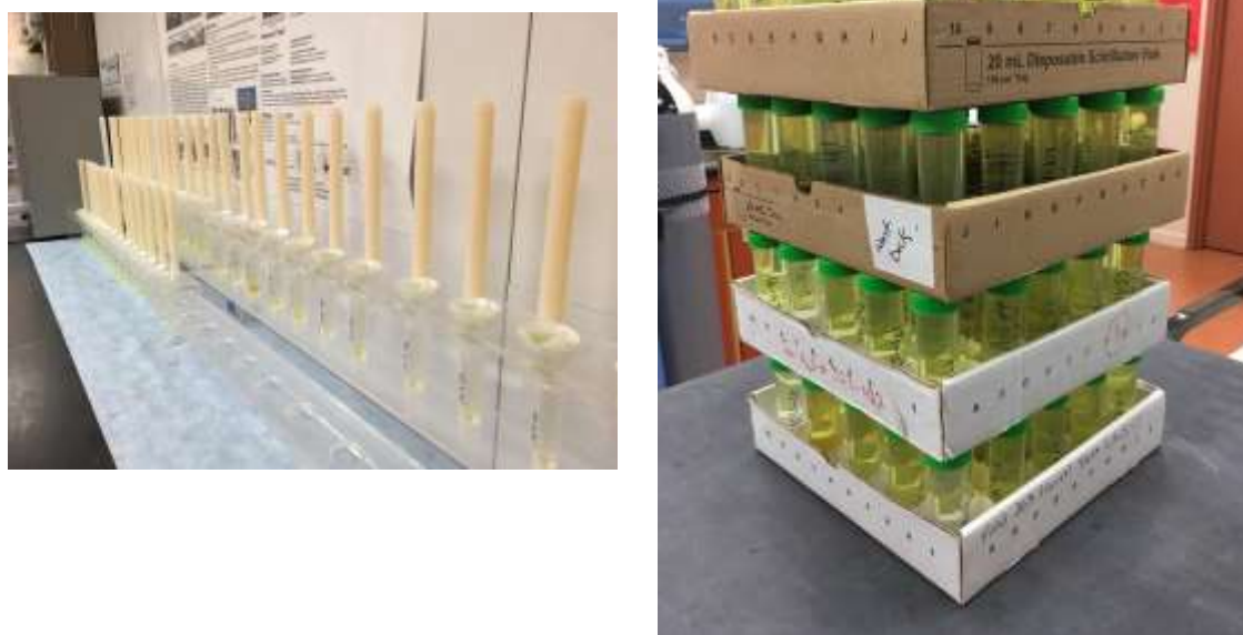
Figure 3. Filtering system used for acid digests (left), and a completed set of diluted samples (right).
