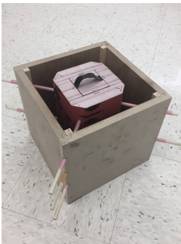
Casting of concrete base and disassembly of the reusable mold
