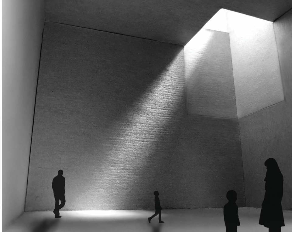
Lighting study: view from within the void at the centre of the mound, with a light well streaming light into the space
