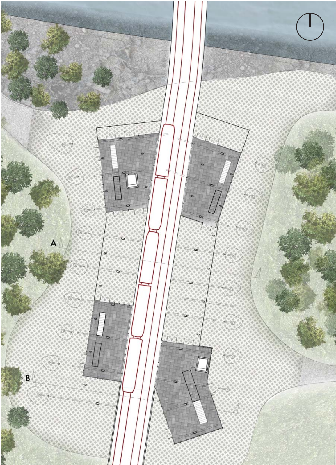
River Valley station main floor plan. The plan adapts to accommodate the existing path system. There are four enclosed spaces for access to the fitness center, and shelter for the transit users.
