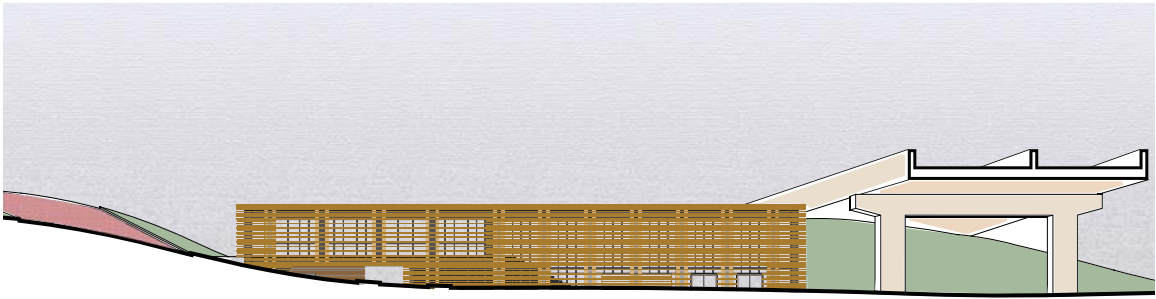
Fig. 93. Section through Site. Screen of building creates a passive presence in the quiet area.
