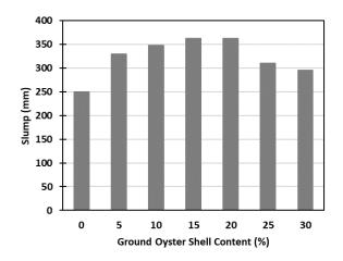
Figure 6: Variation of mini slump for constant water
