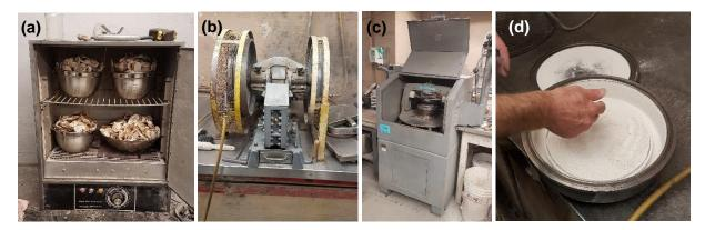
Figure 2: Ground oyster shell preparation: (a) shells are washed and dried; (b) shells are then put through jaw crusher twice; (c) shells are run through the pulverizer for 4 minutes; and (d) final oyster shell product
