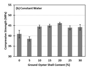
Figure 5: Variation of compressive strength: (a) constant slump mixes and (b) constant water mixes
