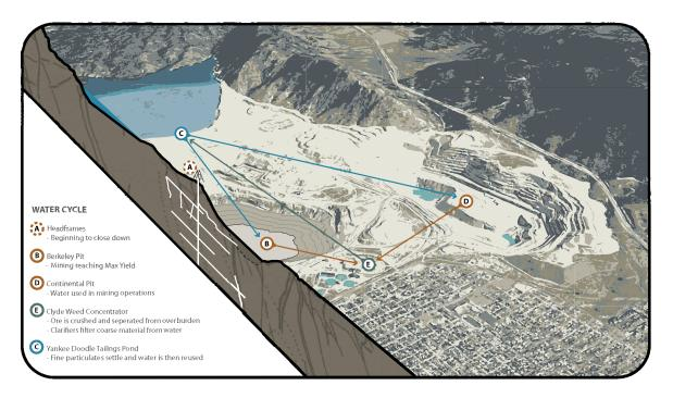
1963 Clyde Weed Concentrator (15 building complex) built in Butte, just South of the Berkeley Pit. Separates waste rock and grinds ore into concentrate before shipping to Anaconda for smelting
