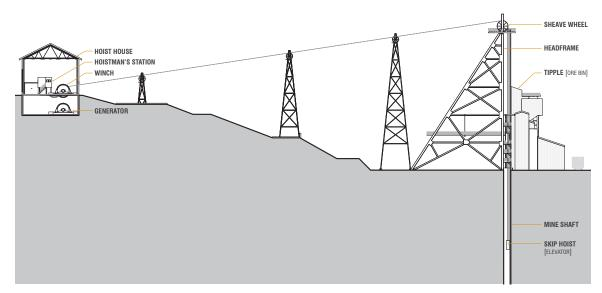
Diagram of the Typical Components of a Headframe Mine in Butte, Montana.
