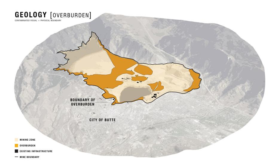
Diagram Showing Where the Topography has been Modified by Mounds of Overburden (Contaminated Waste Soils).
