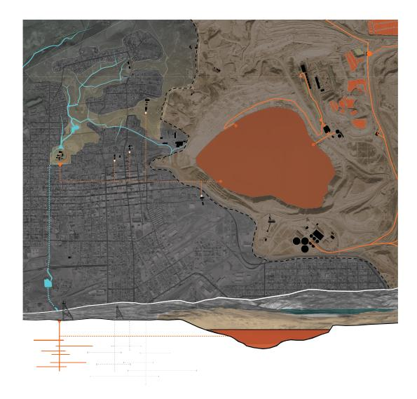
Underground Tunnels Connecting the Headframes with the Water from the Berkeley Pit. Water from the Pit may be Pumped from these Remote Locations within the City.
