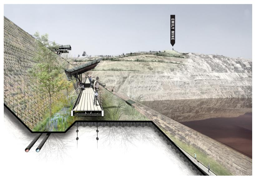
Section Perspective Through the Slope Stabilization Swale and Boardwalk.
