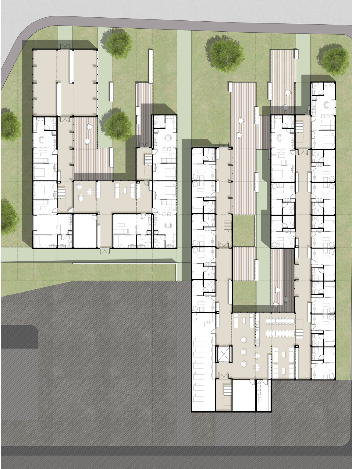
School street proposed building- Main floor plan consisting of mainly smaller single room units for older more dependant residents. Shared kitchen and laundry as well as a small clinic. Some loosely programmed common space along the peripheries of the project for annual activities that could spill out into the courtyards created by the juxtaposition of porous blocks. Emphasis on intersections of public and private space.
