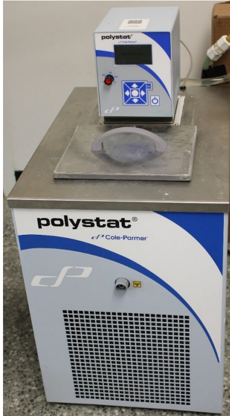
Figure 2.4: Cole-Parmer Polystat RK-12122-52 15L 230 V circulating bath
