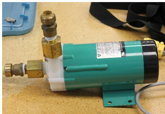
Figure 2.5: Picture of an Iwaki MD-30RT-115NL pump
