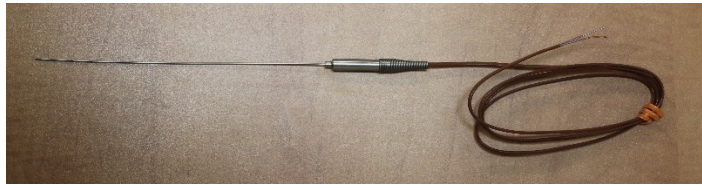
Figure 2.6: Photograph of a T-type thermocouple probe with special limits of error
