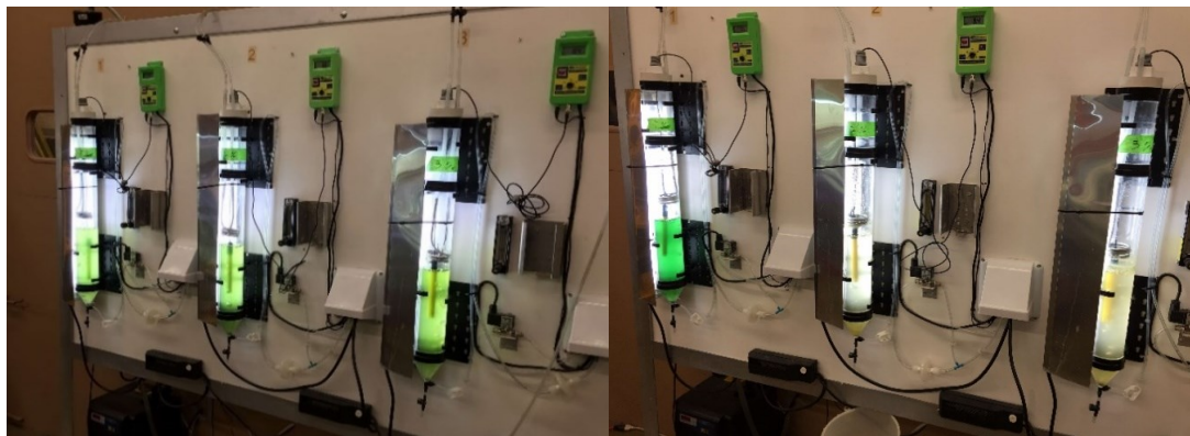
Figure 3.2. Chlorella vulgaris (left) and Anabaena sp. (right) cultivated in the 1, 2, and 3% pre-treated minkery wastewaters, respectively.
