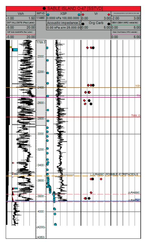
Figure D-3: Sable Island O-47 well section of the Jurassic interval.
