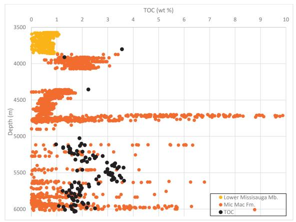
Figure 4-6: Calculated TOC estimates in the shales of South DesBarres O-76.
