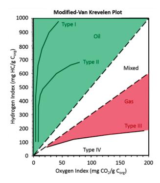
*Figure 1-2: Modified Van Krevelen plot outlining the separation of kerogen and hydrocarbon type (modified from Tyson 1995).*
