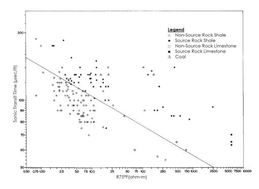
Figure 3-8: Cross-plot of sonic transit time versus resistivity at 75° F (23.9° C) consisting of samples from prolific source rocks from 15 wells located in 9 different countries (Meyer et al. 1984).
