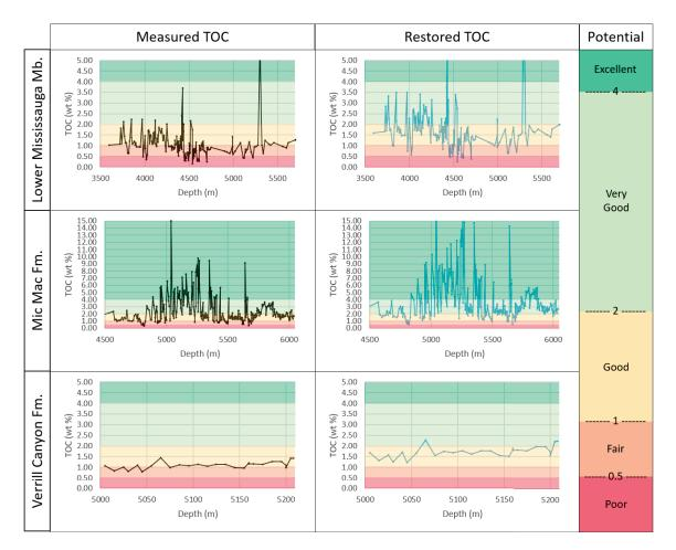
*Figure 4-2: Source rock potential of the 11 key wells separated by formation and TOC Type (based on designations by Peters et al. 2005).*
