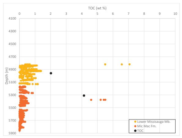
Figure 4-10: Calculated TOC estimates in the shales of Venture B-43.
