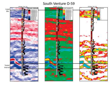
Figure 4-28: Seismic Inline surrounding the South Venture O-59 well, highlighting A) the original seismic data, B) the inverted seismic, and C) the TOC profile.
