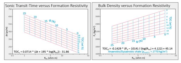
*Figure 3-7: Formation resistivity vs sonic and resistivity vs bulk density cross-plots (modified from Issler et al. 2002).*
