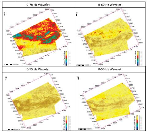
Figure H-6: Cross correlation of the synthetic seismogram versus the original seismic at a time slice of 3 second. Yellow colors are highly correlated and colder colors indicate a lower correlation.
