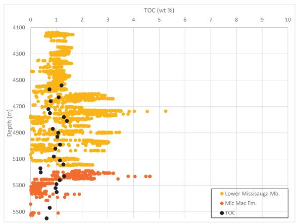
*Figure 4-13: Calculated TOC estimates in the shales of West Venture N-91.*
