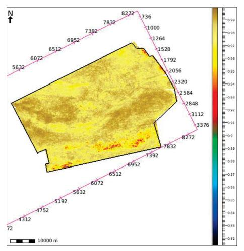
Figure 4-23: Cross-correlation of the synthetic seismogram used to create the inverted seismic versus the original seismic at the 3s interval, all areas are correlated above 0.9 (90%).
