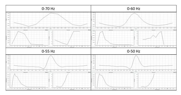
*Figure H-2: Multi-well wavelet for each bandwidth with their corresponding amplitude and phase spectra's.*
