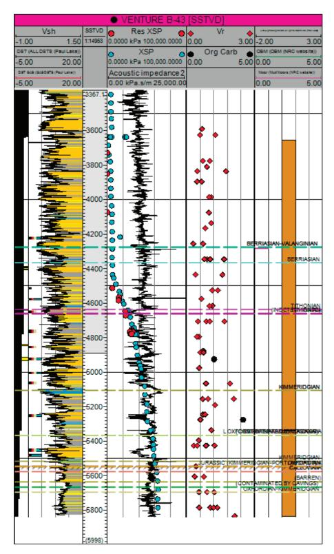
Figure D-8: Venture B-43 well section of the Jurassic interval.
