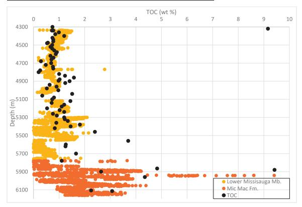
Figure 4-8: Calculated TOC estimates in the shales of South Venture O-59.
