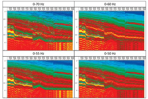
*Figure H-4: Results of the AI inversion over IL 6000 using the four tested wavelets.*
