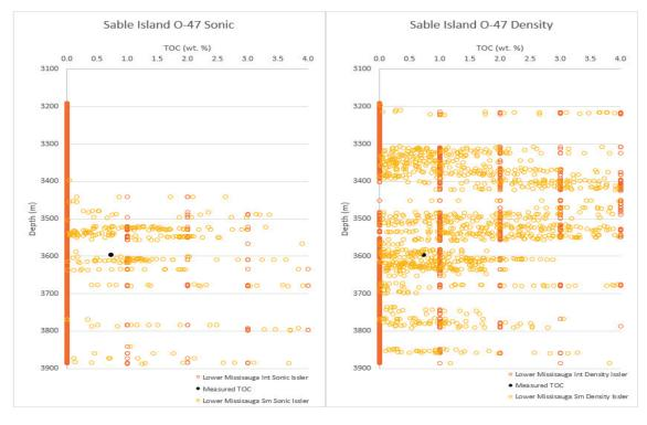
Figure G-3: Unaltered Issler Method results from Sable Island O-47.
