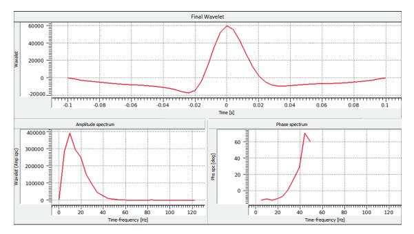
*Figure 4-20: Derived wavelet used in the final inversion with its corresponding amplitude and phase spectra.*
