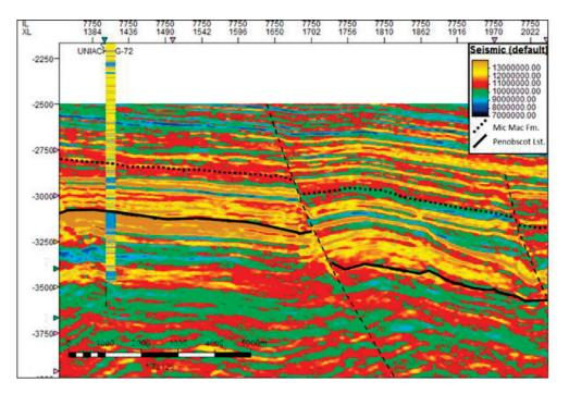
*Figure 5-4: AI inversion cross-section of Inline 7750 highlighting the top of the Mic Mac Formation (black dotted line) and the top of the Penobscot Limestone (solid black line).*
