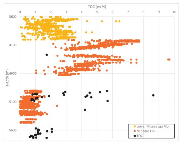
Figure 4-9: Calculated TOC estimates in the shales of Uniacke G-72.
