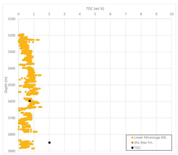
Figure 4-5: Calculated TOC estimates in the shales of Sable Island O-47.
