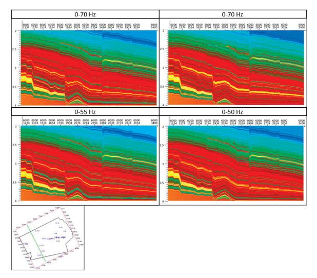
*Figure H-3: Comparison of A-Priori models created from each of the four tested wavelets.* With these steps completed, the four test inversions were run. The inversion parameters used with each tested wavelet. The QC parameters used in each inversion can be seen in Table H-3. The merge cut-off frequency was kept at the default 6 Hz.
