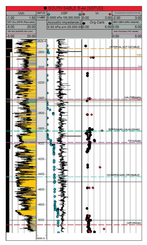
Figure D-5: South Sable B-44 well section of the Jurassic interval.
