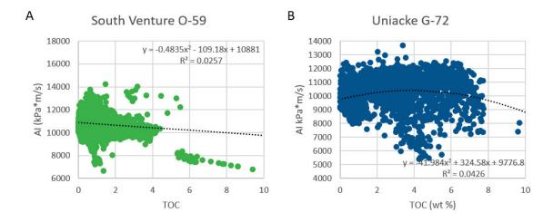
Figure 4-25: Acoustic impedance versus TOC cross-plots for the shales in A) South Venture O-59 and B) Uniacke G-72 for the inverted interval.
