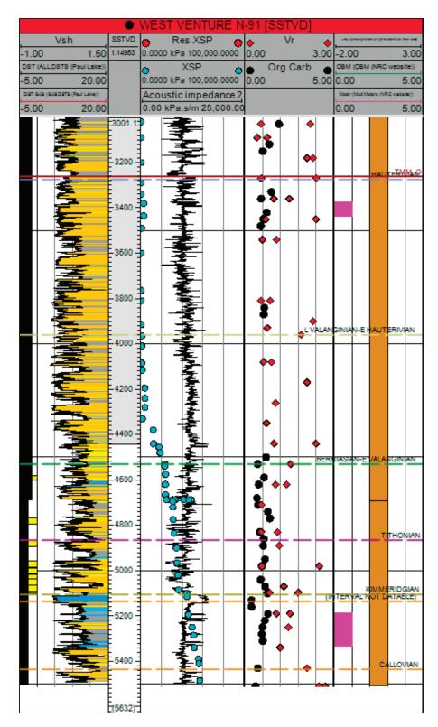
Figure D-11: West Venture N-91 well section of the Jurassic interval.
