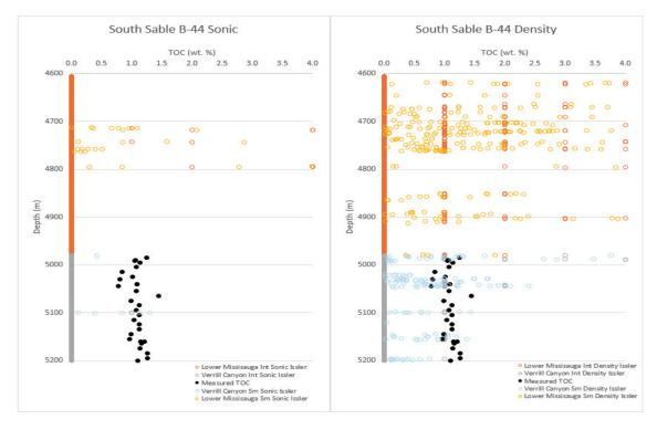
Figure G-5: Unaltered Issler Method results from South Sable B-44.
