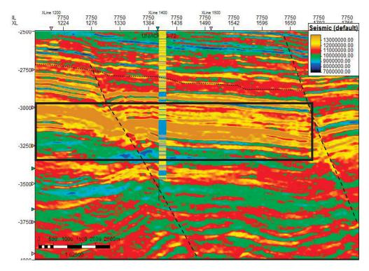
Figure 5-3: Acoustic Impedance inversion cross-section of Inline 7750 highlighting the high impedances of the Penobscot Limestones and their agreement with the limestones highlighted by the CanStrat lithology logs.
