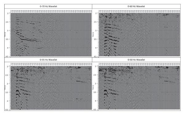
*Figure H-7: Residuals created during the inversion. Dark wiggles indicate a high residual and straighter represent low residual.*
