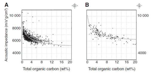
Figure 3-12: Cross-plots of Acoustic Impedance vs TOC depicting a clear non-linear relationship in A) the Kimmeridge Clay, southern England, and B) the Hekkingen Formation in the Barents Sea.
