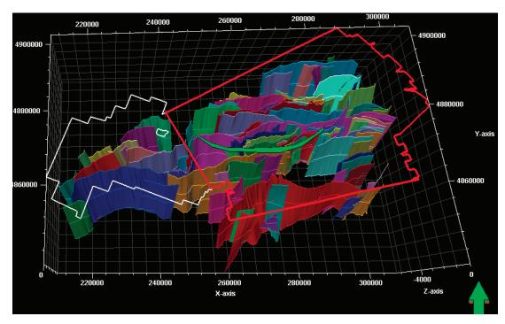
Figure 4-16: 3D view of fault model with the Sable MegaMerge outlined in white, the study area outlined in red and Sable Island shown in green.
