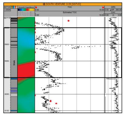
Figure 4-26: Well section of the South Venture O-59 well, outlining the correlated area in black, where increases in TOC correspond to lower AI values and higher estimated TOC values.
