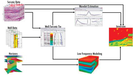
*Figure 3-10: A schematic of the InverTrace*<sup>*PLUS</sup> <i>seismic inversion process (modified from Fugro-Jason 2013).*</sup>
