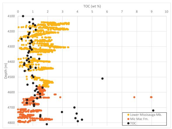
Figure 4-12: Calculated TOC estimates in the shales of West Olympia O-51.
