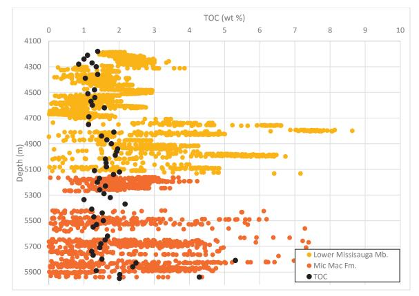
*Figure 4-11: Calculated TOC estimates in the shales of Venture B-52.*
