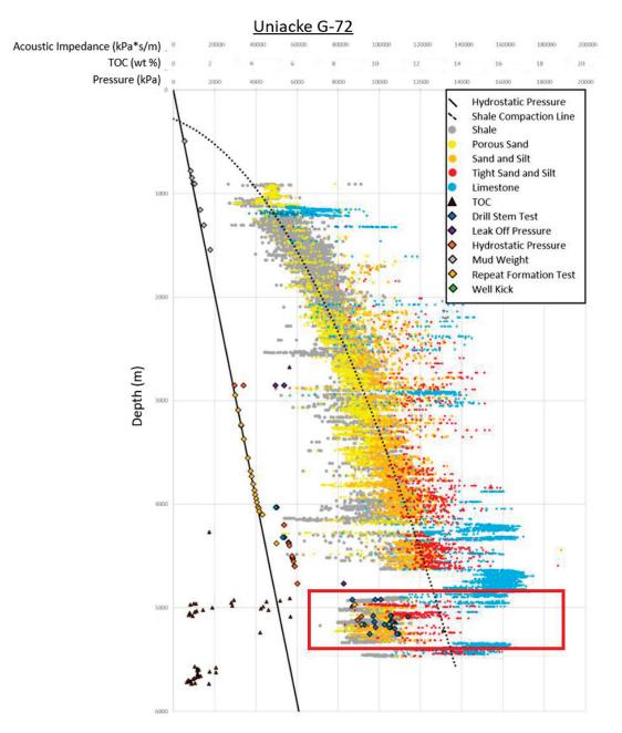
*Figure 5-8: Cross-plot of AI, TOC and pressure measurements versus depth. The red box shows the interval of low AI that corresponds with excess pressure values.*
