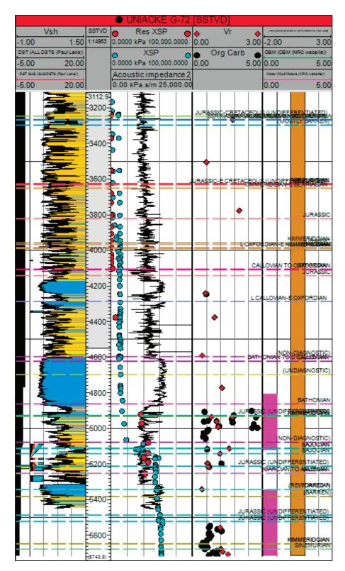
Figure D-7: Uniacke G-72 well section of the Jurassic interval.
