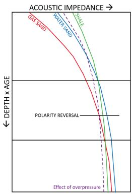
Figure 3-9: Changes in acoustic impedance of shale, wet sand and reservoir with depth and overpressure (modified from Brown 2004).
