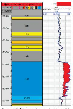
Figure 5-1: Limestone interval with Mic Mac Formation of the Uniacke G-72 well illustrating anomalous ΔLogR values in carbonate intervals due to increased resistivity.
