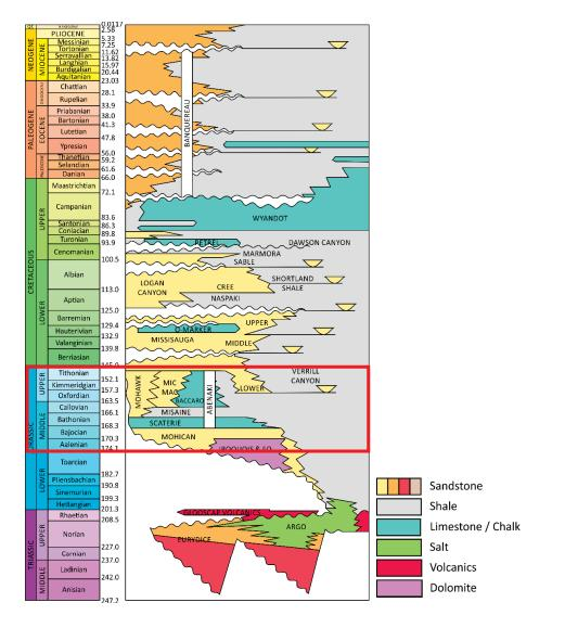
*Figure 2-1: Lithostratigraphic column of the Scotian Basin. Formations of interest outlined in red (modified from Weston et al. 2012).*
