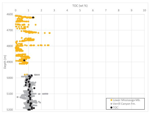
Figure 4-7: Calculated TOC estimates in the shales of South Sable B-44.
