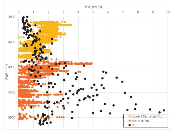
Figure 4-4: Calculated TOC estimates in the shales of Olympia A-12.
