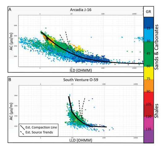
Figure 4-14 Sonic-resistivity cross plots, colored per gamma ray API values for the (A) Arcadia J-16 and (B) South Venture O-59 wells. The solid black like represents the regression or wet, compacted sediment line while the dashed lines indicate possible trends any high TOC point would likely follow.
