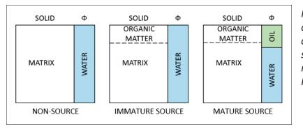
Figure 3-4: Schematic depicting fluid and solid components in both source and non-source rocks (modified from Passey et al. 1990).
