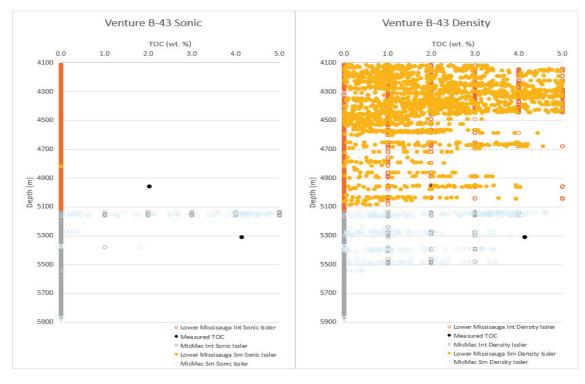
Figure G-8: Unaltered Issler Method results from Venture B-43.
