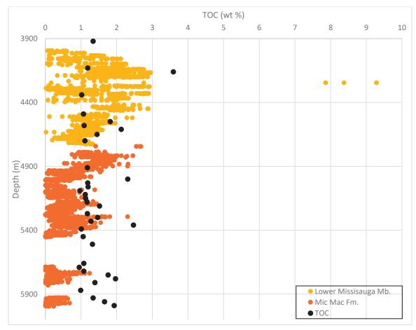
Figure 4-3: Calculated TOC estimates in the shales of Arcadia J-16.
