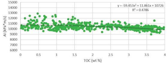
*Figure 4-27:Acoustic impedance versus TOC cross-plot from the shales in South Venture O-59 between 5850-6000 m TVDSS.*
