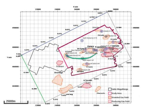
Figure 3-1: Sable MegaMerge 3D Seismic Survey framework, outlining the study area, wells used in the study, and local gas fields.
