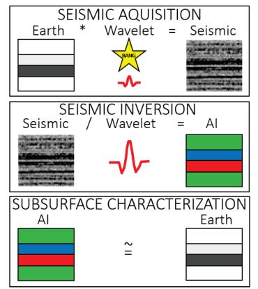
*Figure 3-11 : The process of seismic inversion where \* represents convolution and / represents deconvolution (modified from Fugro-Jason 2013).*
