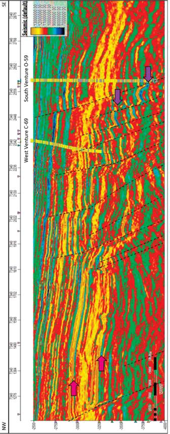
Figure 5-6: Acoustic impedance cross-section of Inline 7340, with the sub-carbonate low impedance intervals identified by the pink arrows and the expansion trend, low-impedance intervals by the purple arrows.
