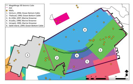
*Figure 1-3: The six 3D seismic surveys included in the Sable MegaMerge survey.*
