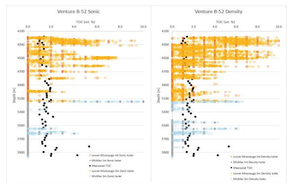
Figure G-9: Unaltered Issler Method results from Venture B-52.
