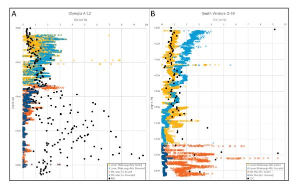
*Figure 5-2: Unscaled vs scaled TOC estimation results for the (A) Olympia A-12 and (B) South Venture O-59 wells providing an example of both adequate and inadequate correlation to measured TOC data.*
