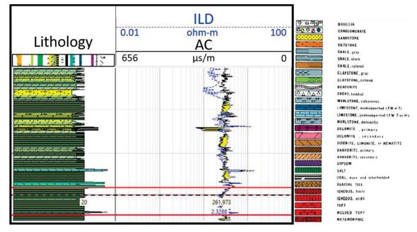
*Figure 3-3: Visual estimation of a sonic and resistivity baselined interval in the South Venture O-59 well with the corresponding sonic and resistivity values.*
