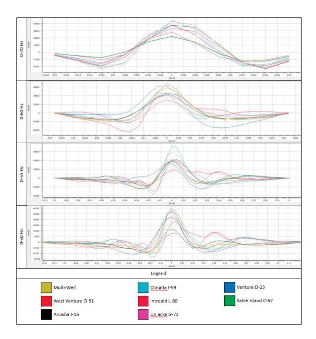
*Figure H-1: Wavelets for each well combined to create the multi-well wavelet for the selected bandwidths.*
