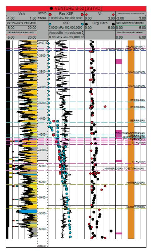
Figure D-9: Venture B-52 well section of the Jurassic interval.
