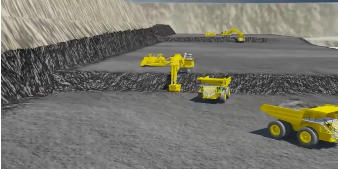
Figure 6.4 Parallel coal shoveling sites (Source: Mycosm - 3D simulation)
