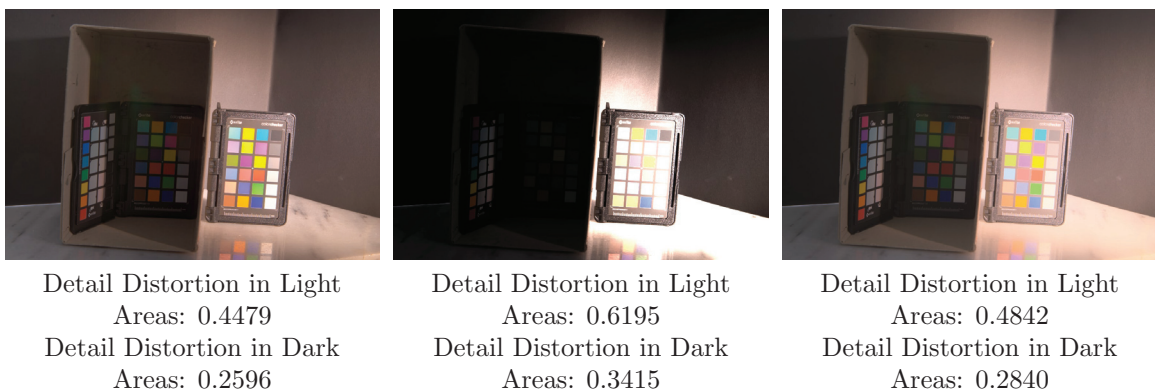
Figure 4.11: Image quality assessment using detail distortion in light and dark areas on the HDR image “Test Chart”. The images are generated from various TMOs with some manipulation of parameter settings. The HDR image is from Empa Media Technology.
