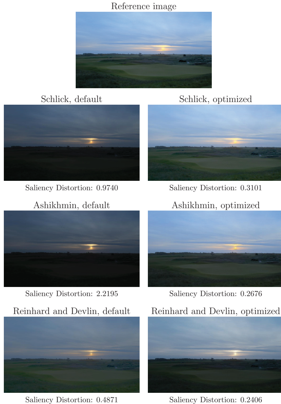
Figure 5.2: Results of the parameter tuning algorithm on HDR image “Bandon Sunset (1)”. Shown are the reference image tone mapped with manual manipulation (provided at [26]), images tone mapped with Schlick’s, Ashikhmin’s, and Reinhard and Devlin’s operators and default parameter settings, and images tone mapped with optimized parameter settings. The HDR image is from Mark D. Fairchild’s HDR Photographic Survey and © 2006-2007 Mark D. Fairchild.
