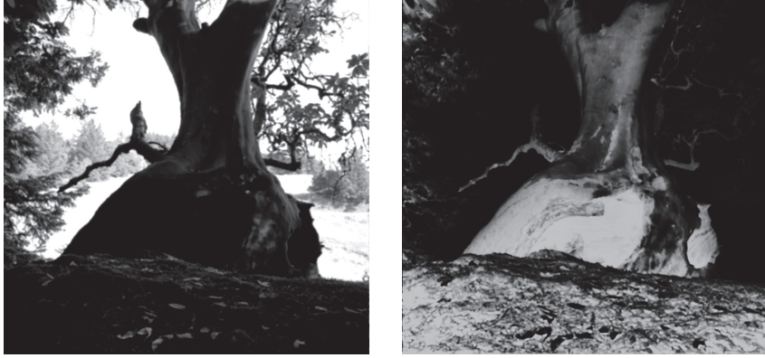
Figure 4.8: Weight maps that represent light (left) and dark (right) areas. The HDR image is from Industrial Light & Magic.
