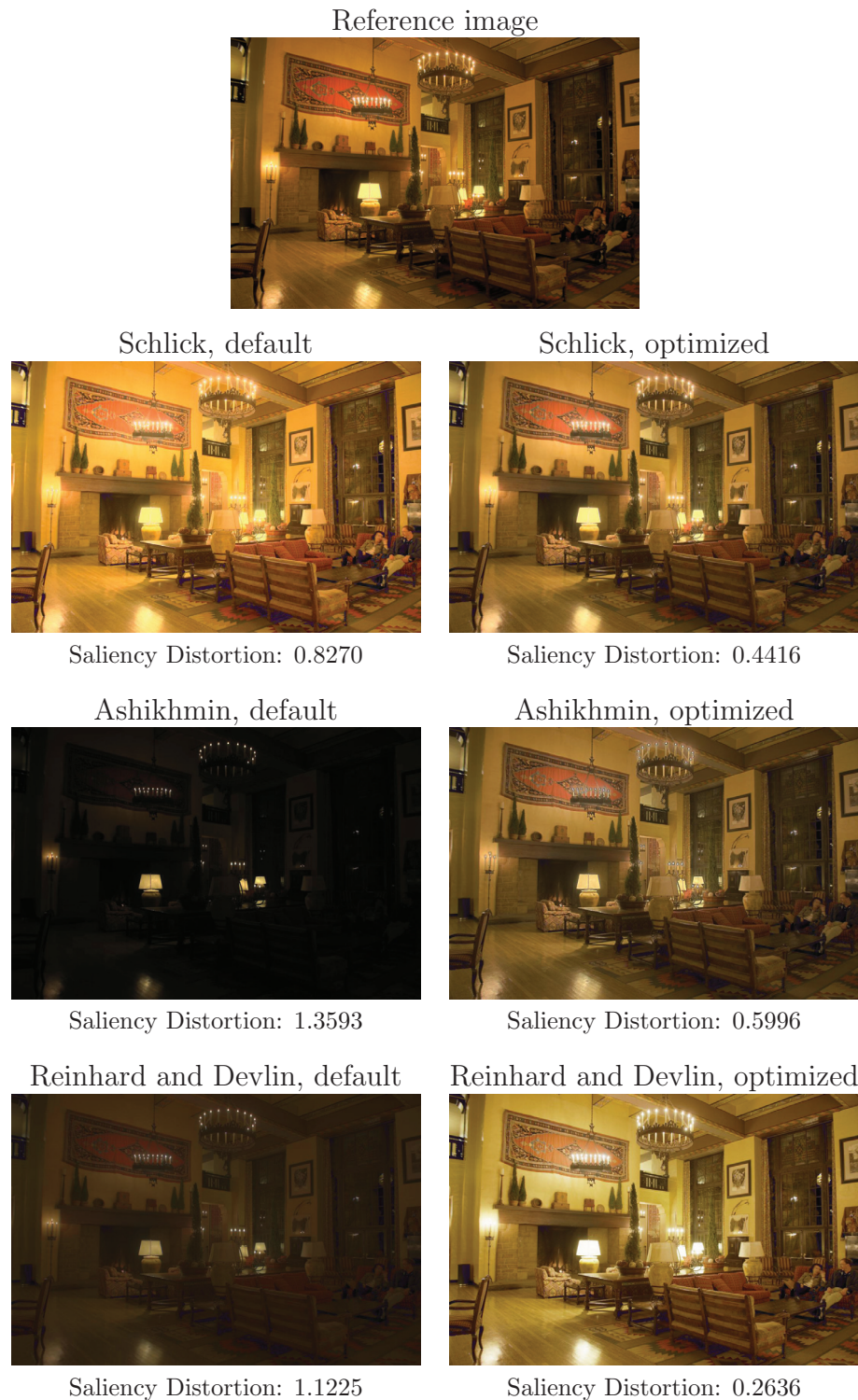
Figure 5.5: Results of the parameter tuning algorithm on HDR image “Ahwahnee Great Lounge”. Shown are the reference image tone mapped with manual manipulation (provided at [26]), images tone mapped with Schlick’s, Ashikhmin’s, and Reinhard and Devlin’s operators and default parameter settings, and images tone mapped with optimized parameter settings. The HDR image is from Mark D. Fairchild’s HDR Photographic Survey and © 2006-2007 Mark D. Fairchild.
