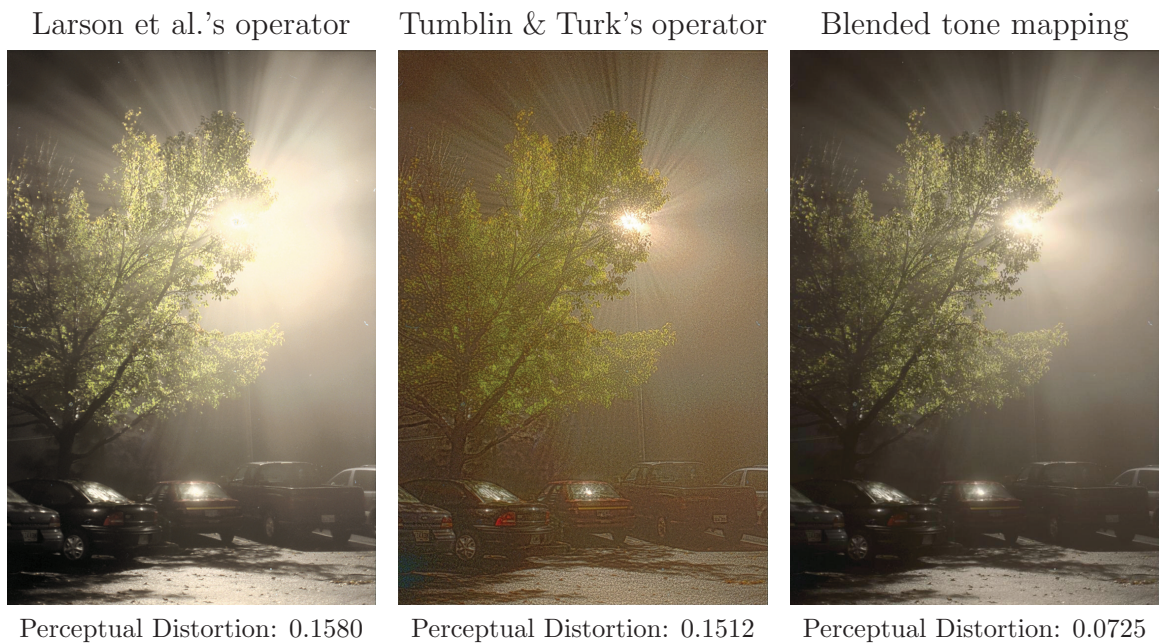
Figure 5.13: Comparison of blended tone mapping with TMOs on HDR image “Foggy Night”. Shown are the tone mapped images generated by Ward et al.’s, and Tumblin and Turk’s operators, and blended tone mapping. The HDR image is from Jack Tumblin.
