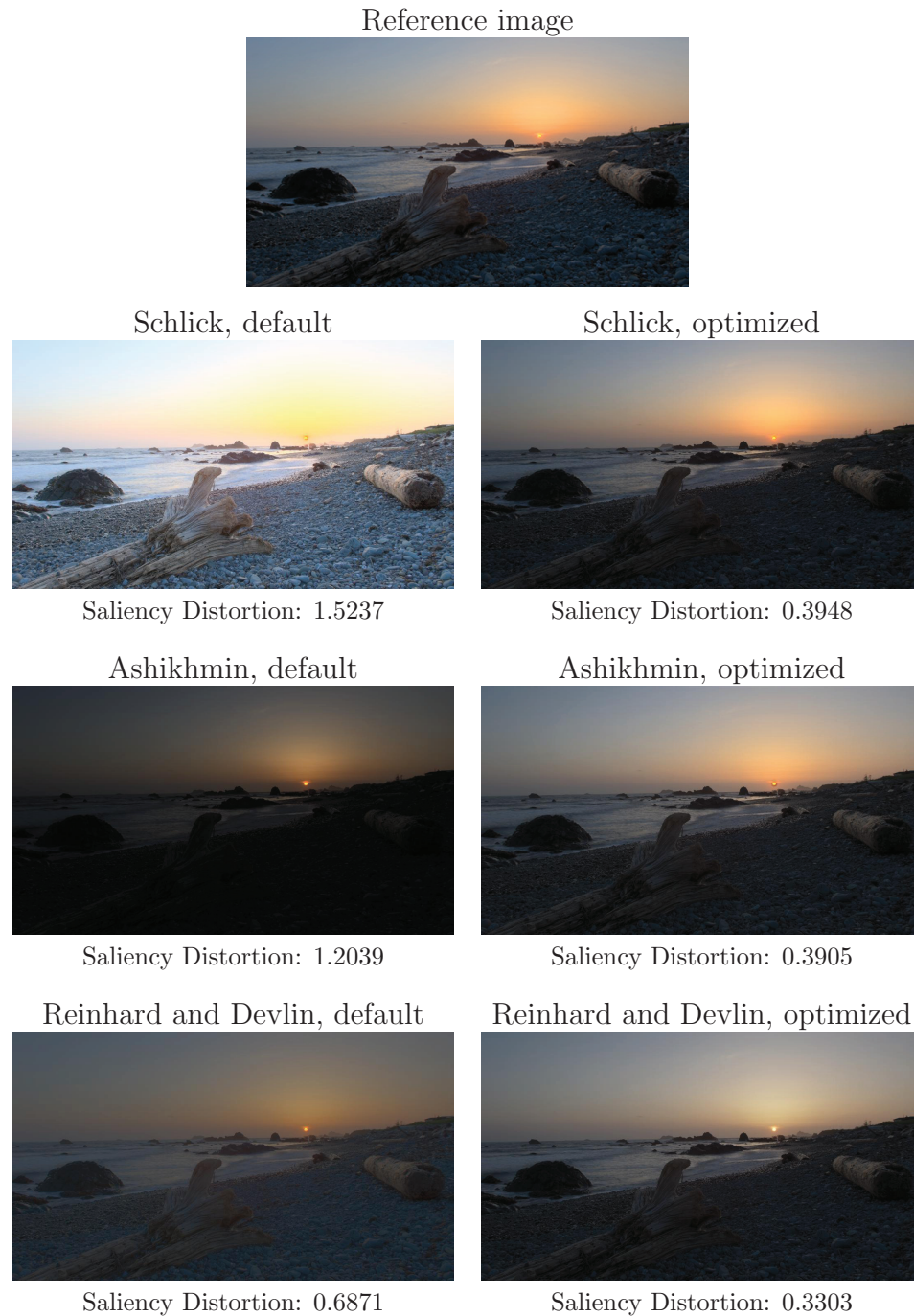
Figure 5.3: Results of the parameter tuning algorithm on HDR image “Redwood Sunset”. Shown are the reference image tone mapped with manual manipulation (provided at [26]), images tone mapped with Schlick’s, Ashikhmin’s, and Reinhard and Devlin’s operators and default parameter settings, and images tone mapped with optimized parameter settings. The HDR image is from Mark D. Fairchild’s HDR Photographic Survey and © 2006-2007 Mark D. Fairchild.
