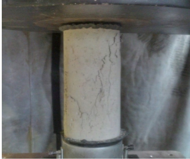
Figure 4.6 Typical Failure Mode of Concrete Cylinder
