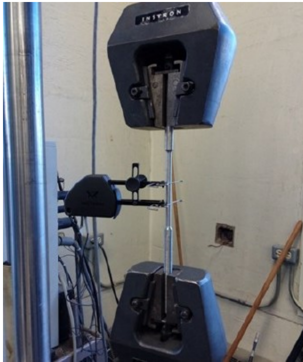
Figure 3.25 Tension Test Set-up for Steel Coupons (Hu 2015)
