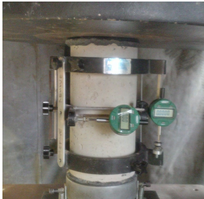
Figure 3.23 Concrete Modulus and Compression Test
