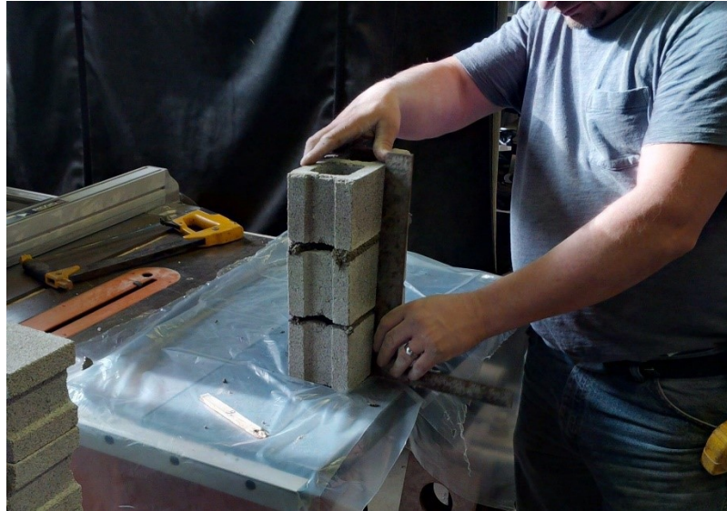
Figure 3.21 Masonry Prism Construction
