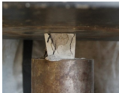
Figure 4.3 Typical Failure Mode of the Mortar Cubes
