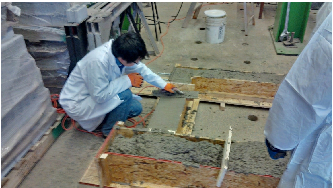
Figure 3.9 Concrete Surface Smoothing with Trowel
