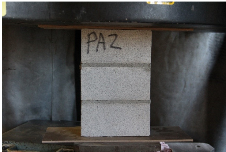
Figure 3.22 Masonry Prism Test
