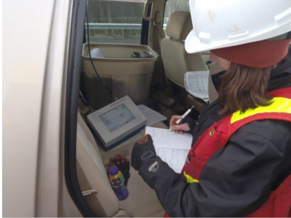
Figure 3.14 Data Logger Indicating Strains on Pile P5N.
