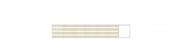
Figure 13. Diagram showing the basic concept of hollow steel sections integrating with CLT panels.
