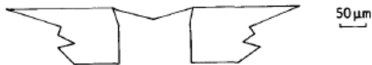
Figure 2.19: Typical Palmqvist crack profile in a cermet [92] .
