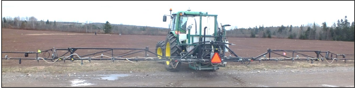
Figure 4-7: Smart sprayer with rear mounted cameras and 27 spray nozzles.
