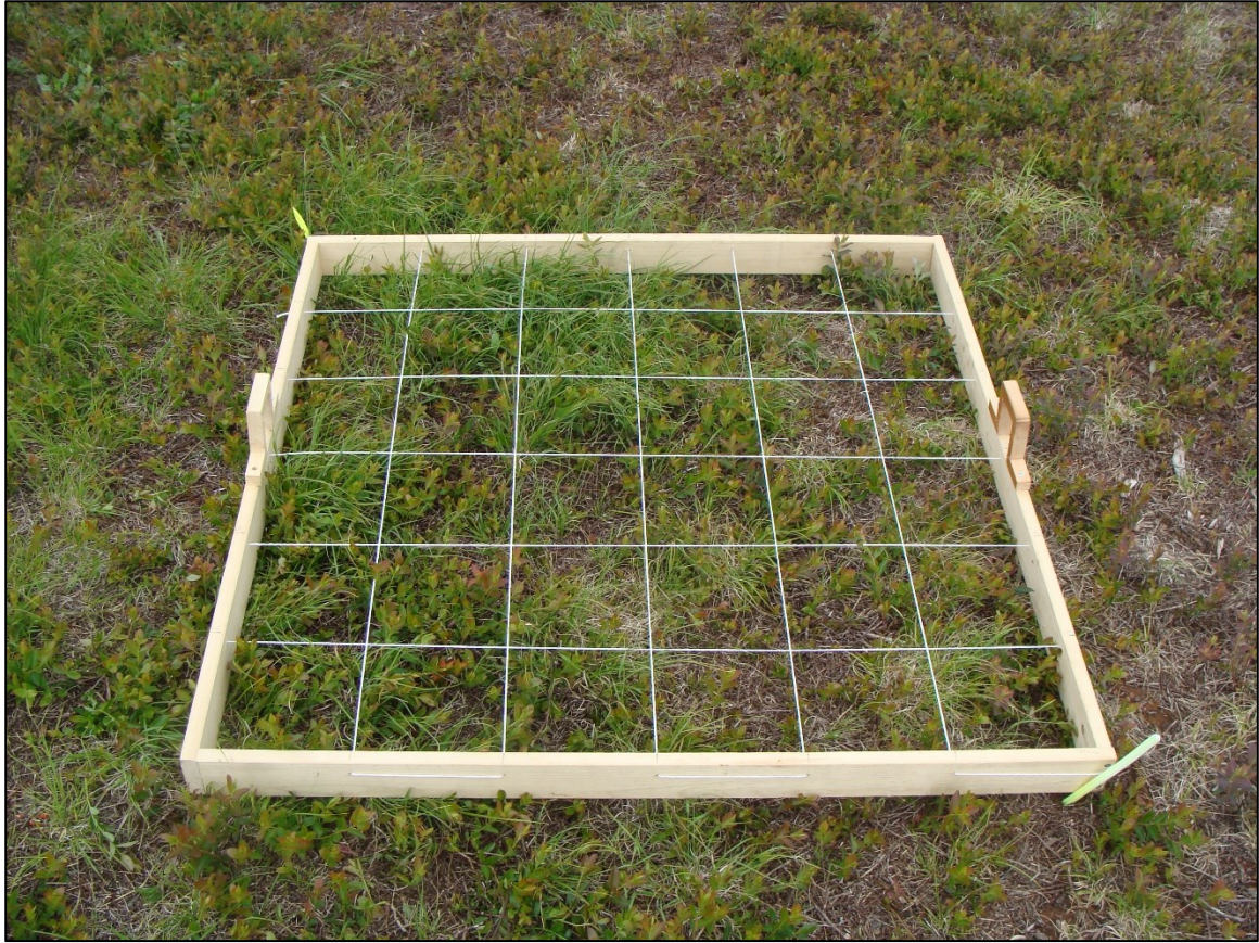
Figure A-11: Square quadrat for determining percent weed coverage from selected plots.
