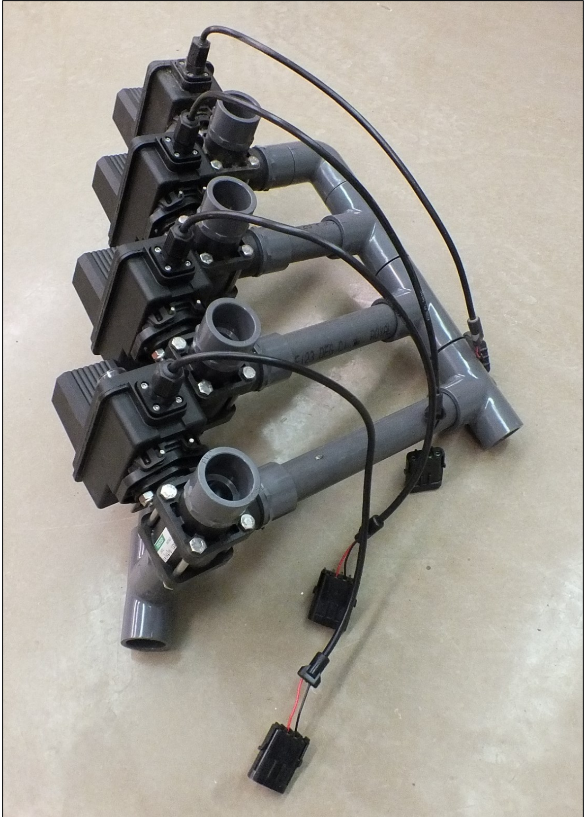
Figure A-2: Custom plumbed flow valve system for boom section control.
