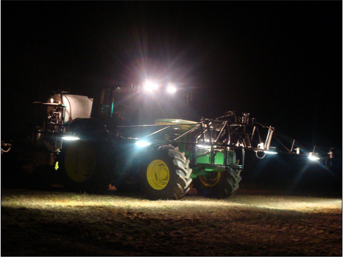
Figure A-14: Machine vision system experimental testing after dark with added light source.
