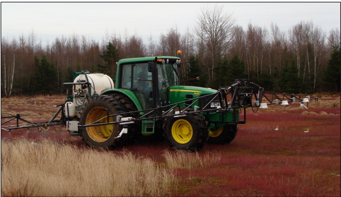
Figure A-10: Herbicide application in selected field with front machine vision boom.
