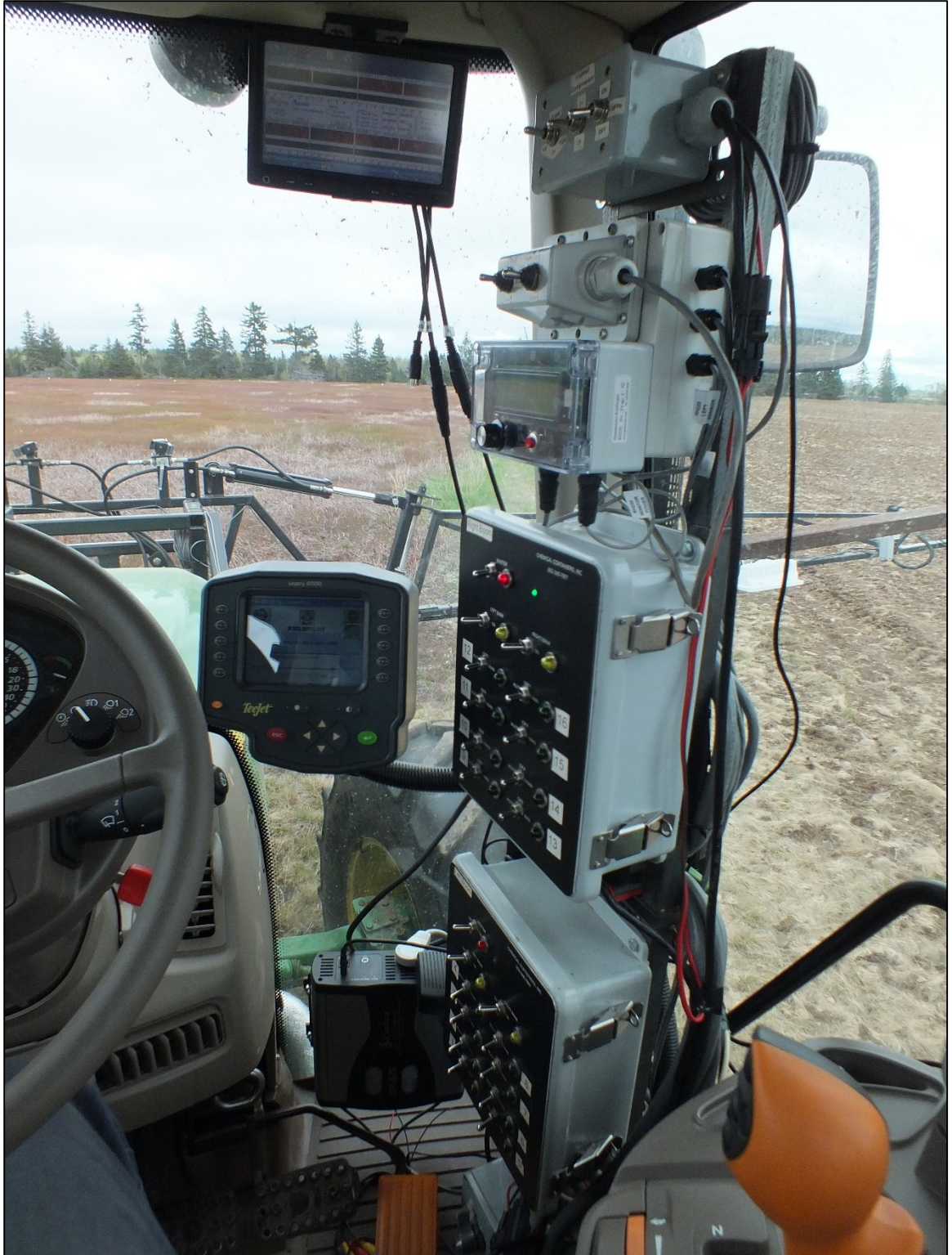
Figure A-6: Operators view of controllers used during initial smart sprayer design and testing.
