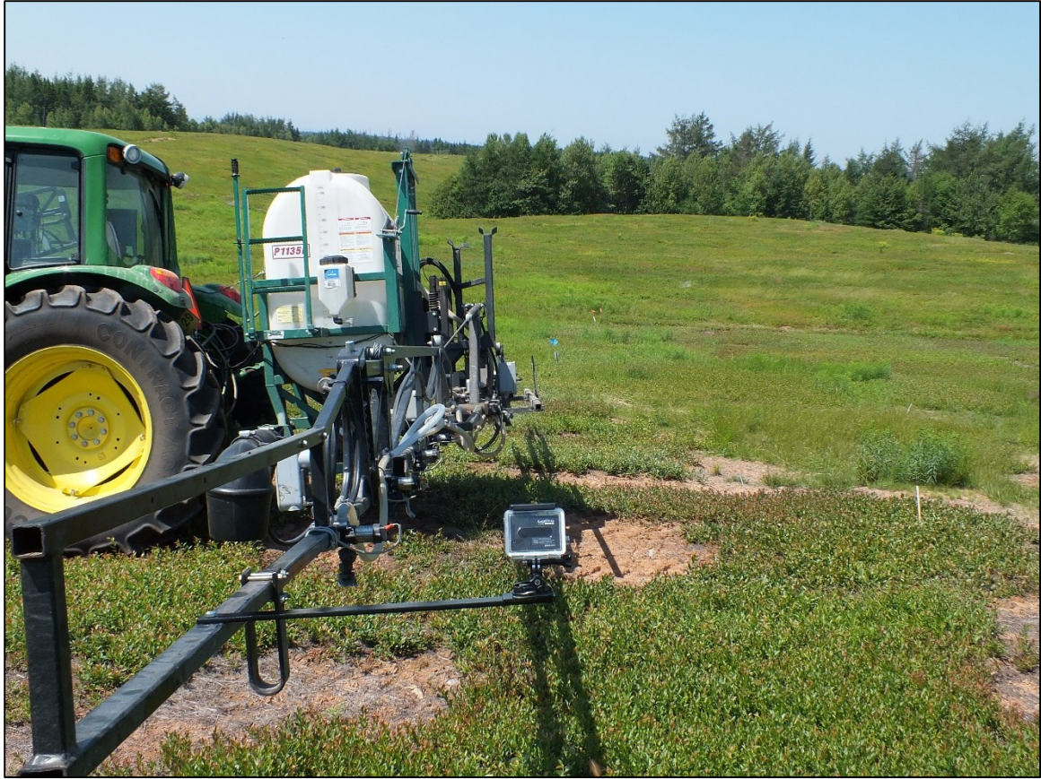
Figure A-16: GoPro® camera mounted on rear sprayer boom for real-time video acquisition during field testing.
