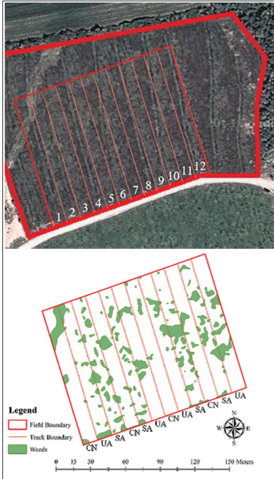
Figure 4-8: East Mines Field aerial photograph (top) showing experimental track setup and GIS map showing moss infected areas (bottom).
