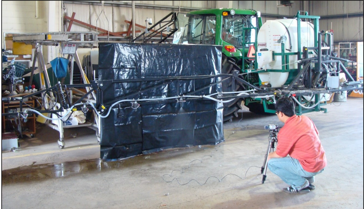
Figure A-4: Experimental setup showing procedure for determination of mechanical delay time.
