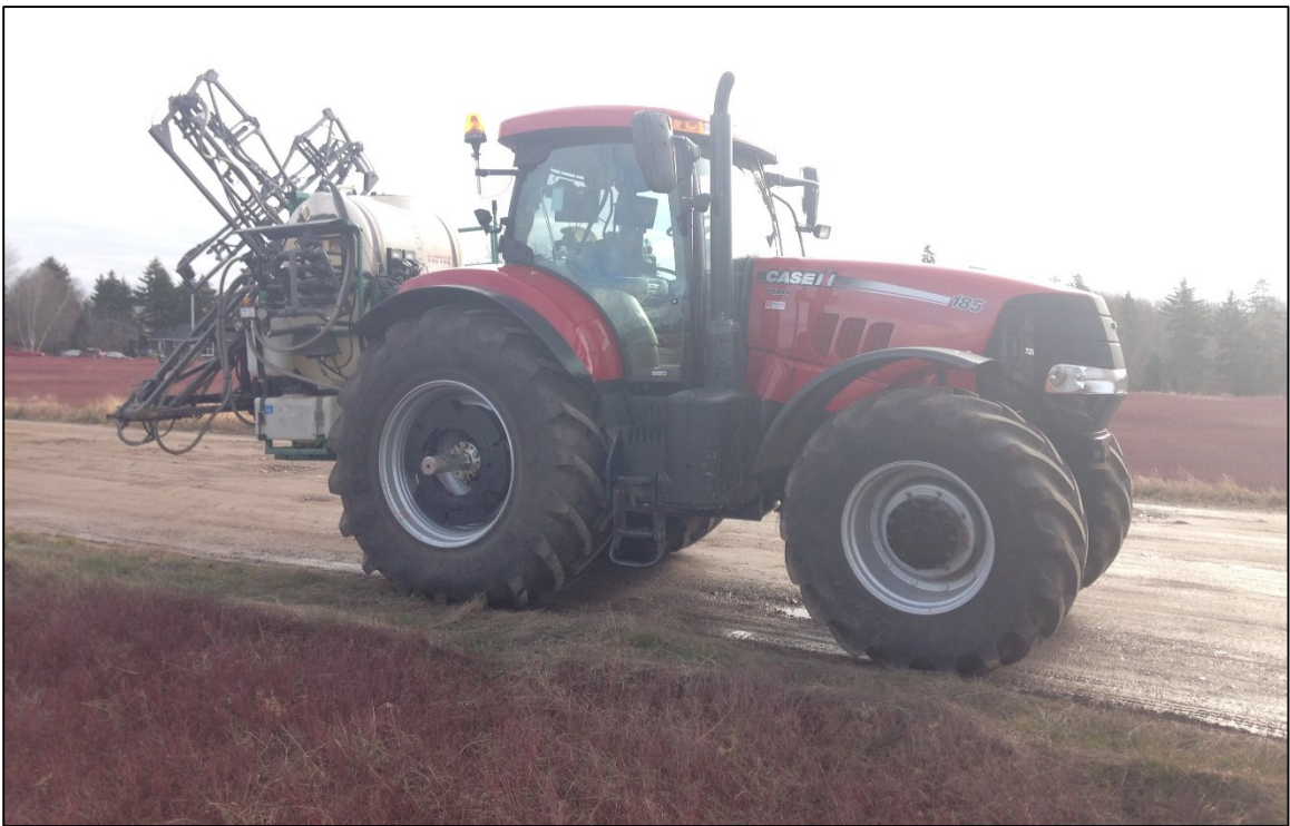
Figure A-18: Field testing smart sprayer system installed on Case 185 farm tractor for spot-application of herbicide.
