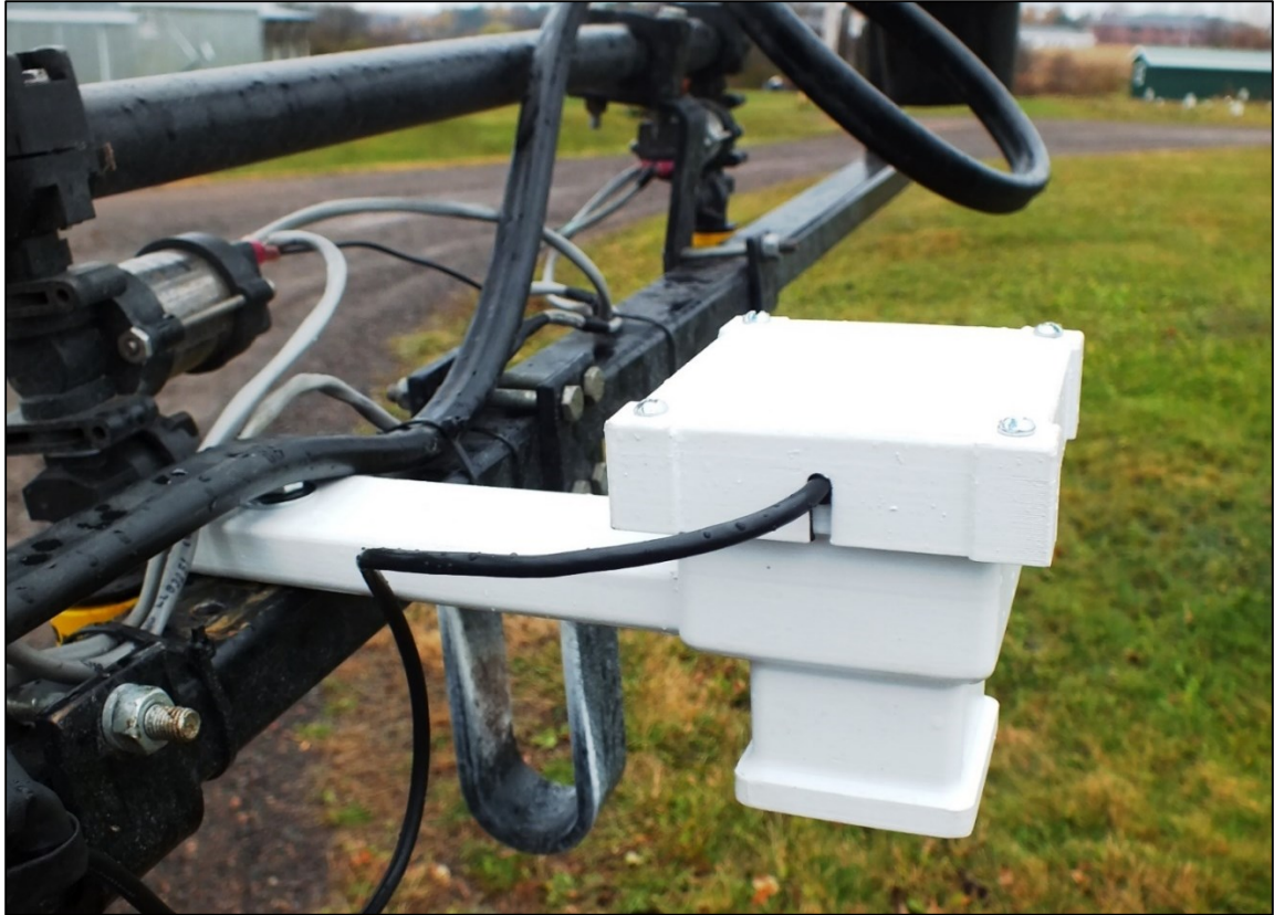
Figure 2-7: Custom made weather resistant smart sprayer camera case painted white and mounted on smart sprayer boom.
