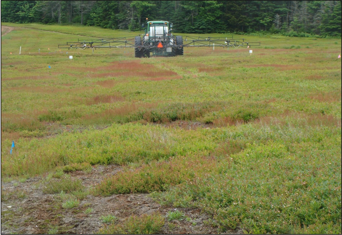
Figure A-9: Fungicide application in selected field using front machine vision system.
