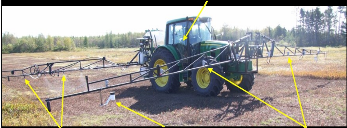
Figure 2-2: The experimental setup showing the cameras out in front of the tractor and the individual nozzle section flow control setup.
