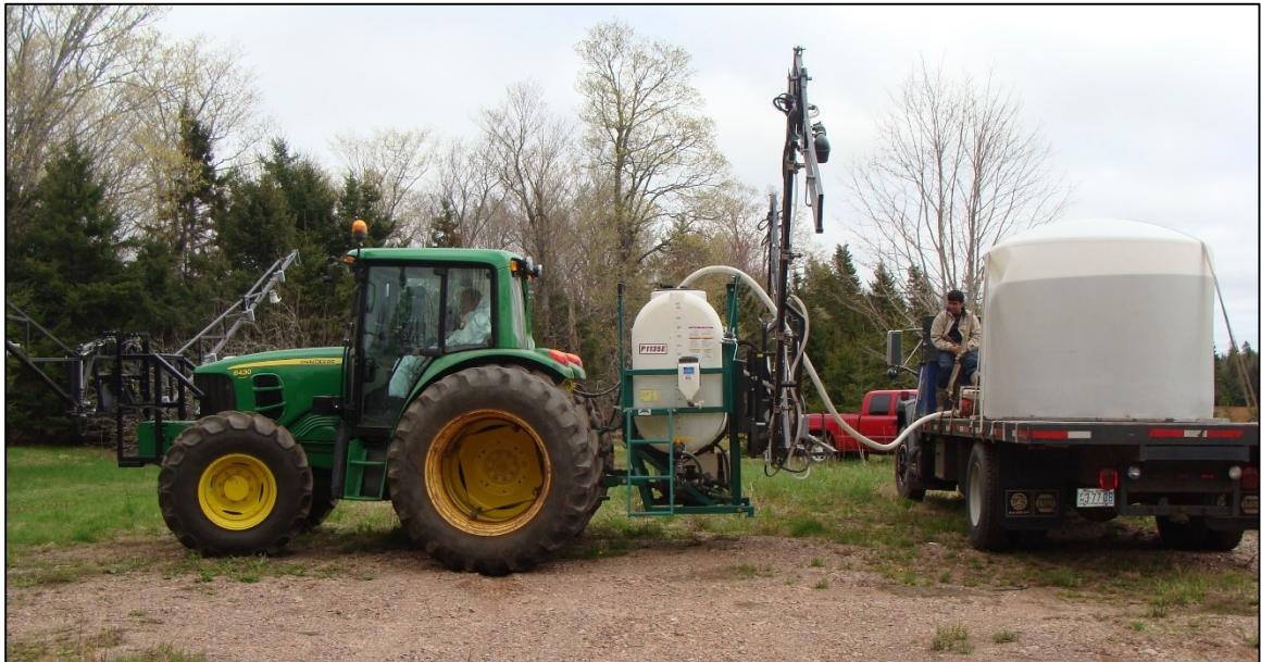
Figure A-8: Smart sprayer tank fill-up using commercial chemical mixing station.
