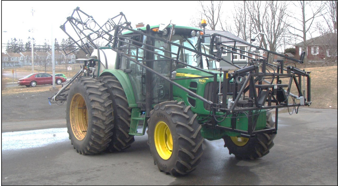
Figure A-7: Front machine vision boom and rear sprayer boom folded in for road travel to research fields.
