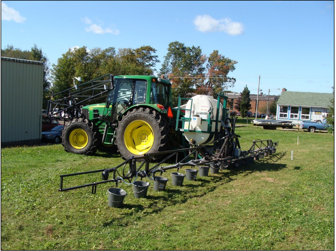
Figure A-3: Flow rate and individual nozzle calibration experimental setup.
