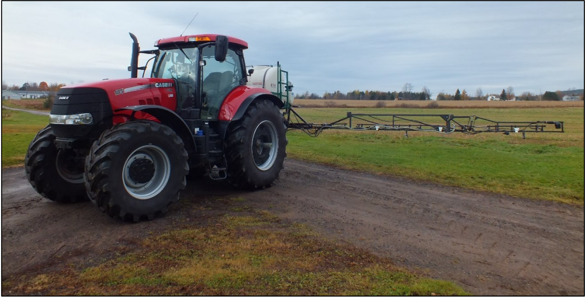
Figure A-17: Refined smart sprayer system installed on Case 185 farm tractor.
