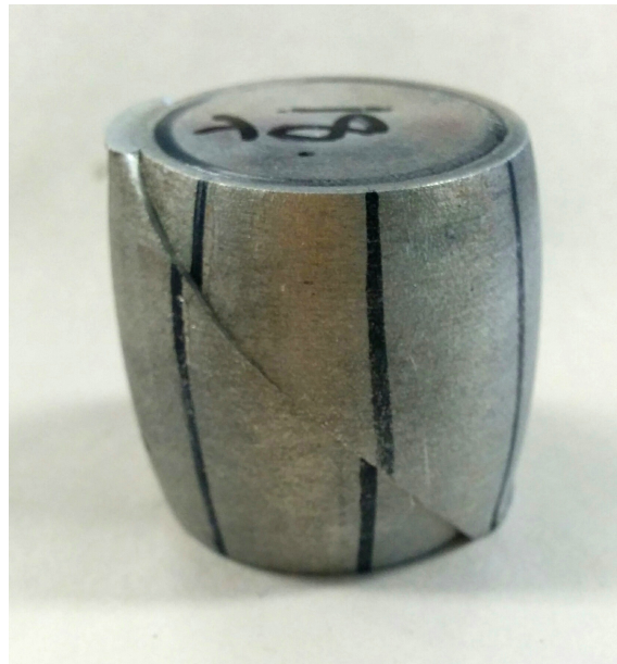
Figure 5.3: Sample 18, with vertical lines showing material movement after fracture
