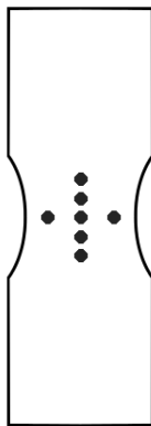
Figure 2.1: Seven dot configuration used in marker-tracking extensometers
