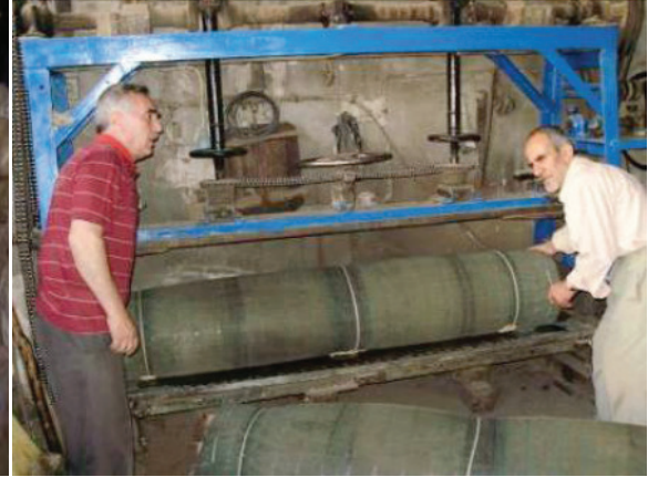
Rolling the wool to put on the felting machine. The felting machine agitates wool.
