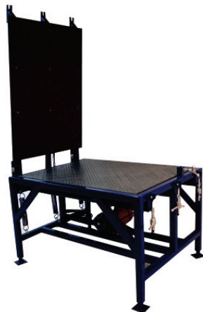
A felting bed (photo from Belfast Mini Mills). A felting loom (photo from feltloom.com).
