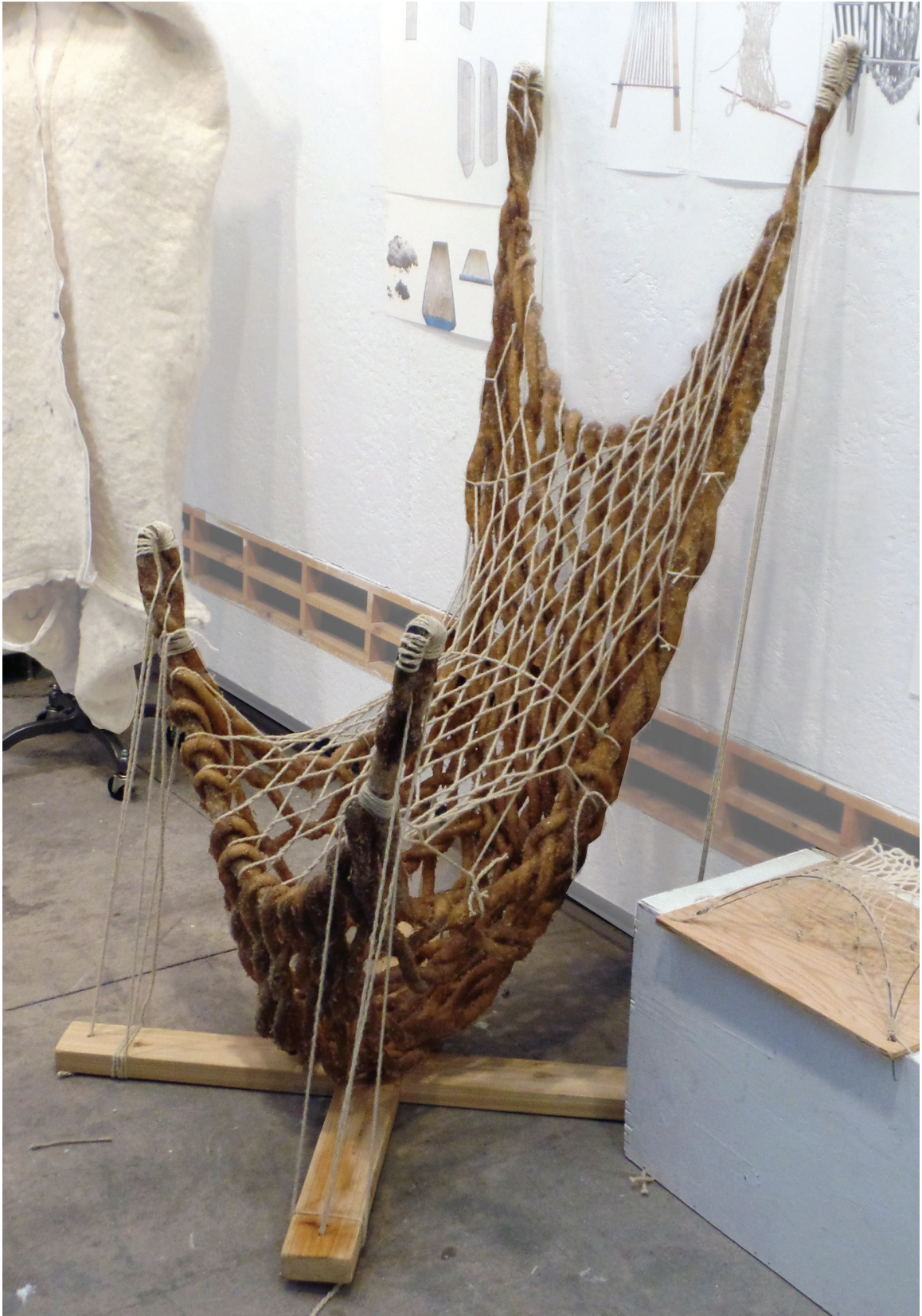
The chair as presented at the thesis defense. When sat it the resin cracks, it has not been tested to see if the cracking will stop and the chair will function.
