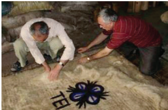
Edges are adjusted, and the front and back of the kepenek are attached with a seam running from the shoulders down the side. The felt is returned to the felting machine.
