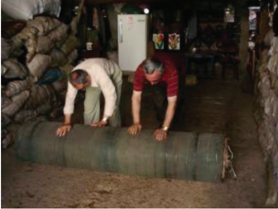
Rolling the wool to put on the felting machine. The felting machine agitates wool.
