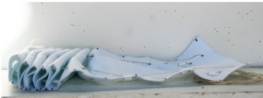
A flimsy piece of felt stands up when it is corrugated.
