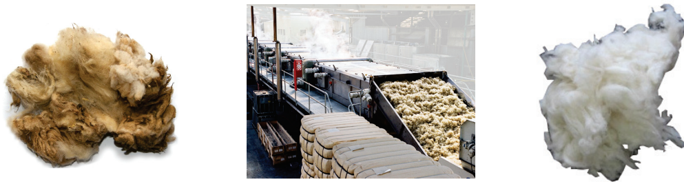
Wool before, during and after scouring (photo from New Zealand Wool Services).
