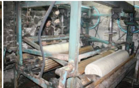
Edges are adjusted, and the front and back of the kepenek are attached with a seam running from the shoulders down the side. The felt is returned to the felting machine.
