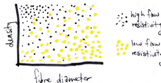
Illustration of flow resistivity as it relates to fabric density and fibre diameter.
